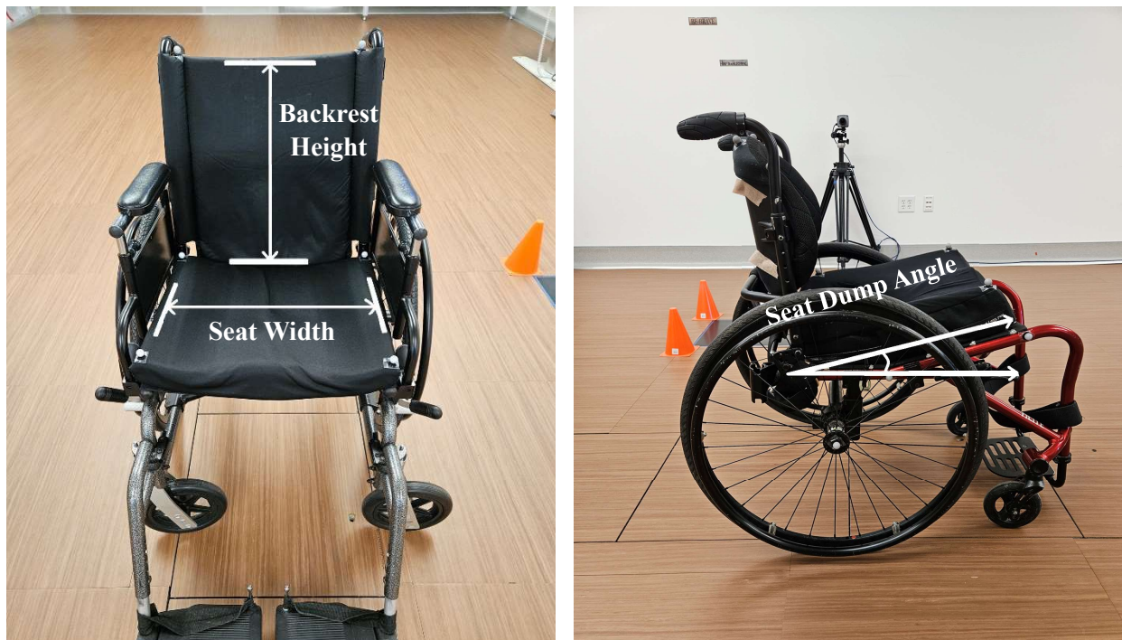
Figure 5: (Left) A front-on view of a wheelchair showing the backrest height and seat width wheelchair variables. (Right) A side-on view of the seat dump angle wheelchair variable.
