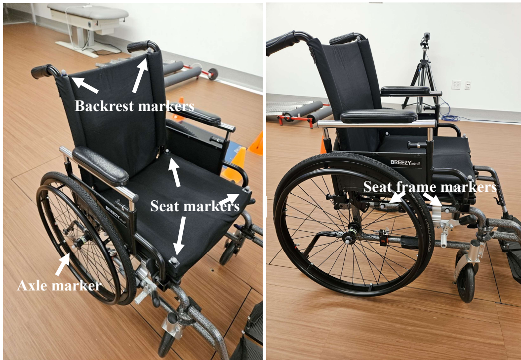
Figure 3: Ten wheelchair markers were used to calculate wheelchair fit measures. The markers are on the backrest, axles, seat, and seat frame.
