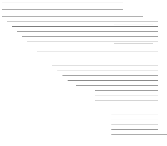
Figure 5-16 Geosynthetic arrangement of the GRS bridge abutment of the 3D bridge system
