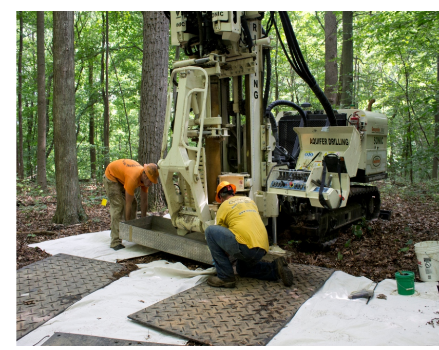
Figure 1 and 2: A track-mounted roto sonic drill was necessary to access roadless areas and minimize environmental impact.
