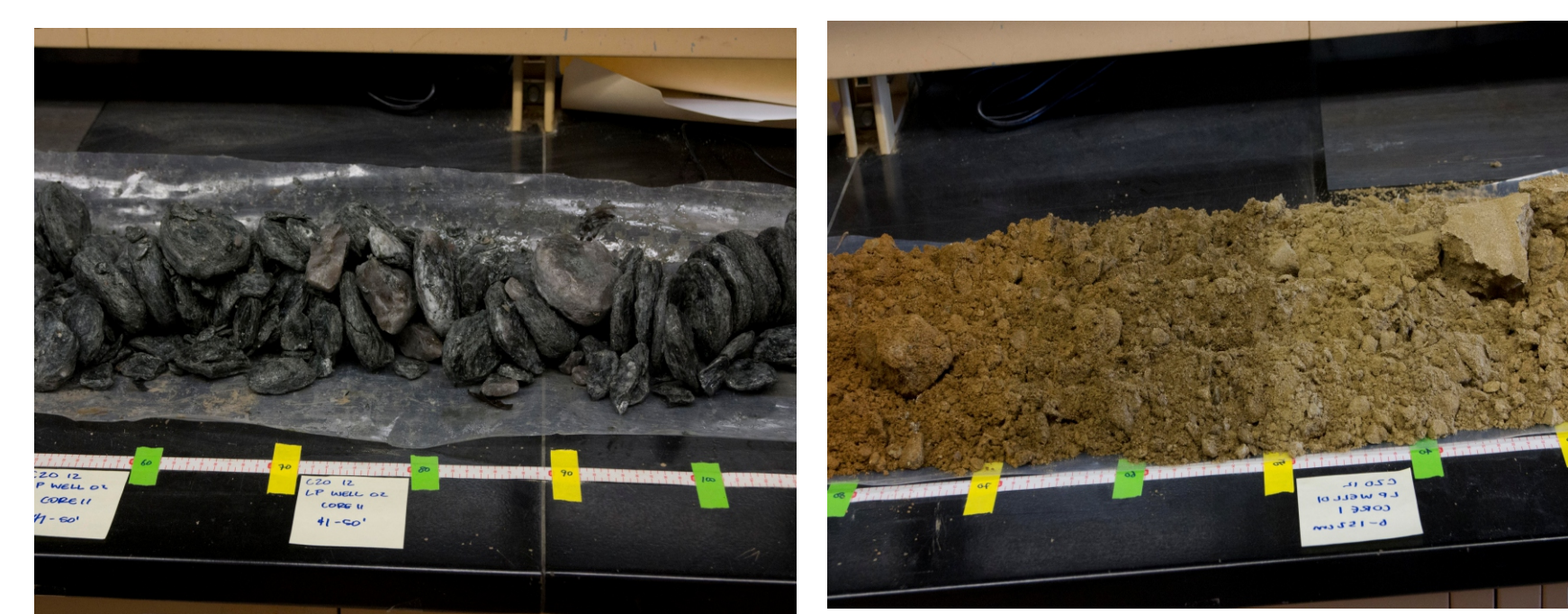
Figure 3: Core drilling yielded a variety of materials, ranging from disaggregated fine sand in the upper portion of the well to fresh bedrock in the lower portion of the well. Note foliated fragments of schist within Well 2.
