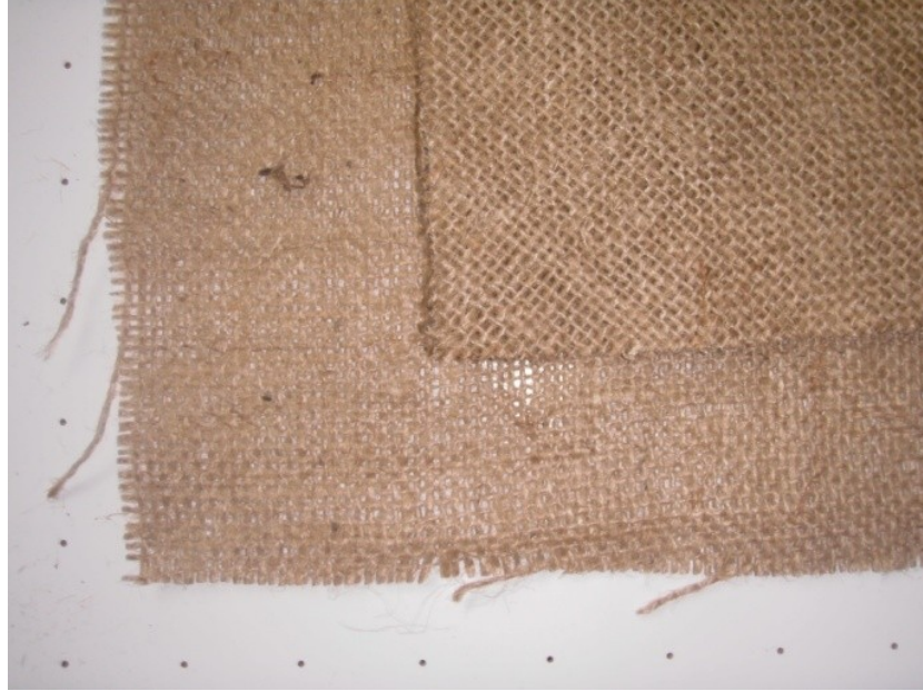
Figure 21: Layup 4 ( 0^{\circ}_A, 45^{\circ}_A ).
