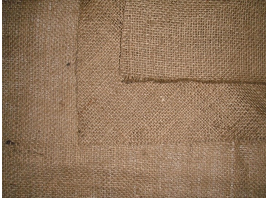
Figure 17: Layup 2 ( 0^{\circ}_A , 45^{\circ}_A , 0^{\circ}_A ).
