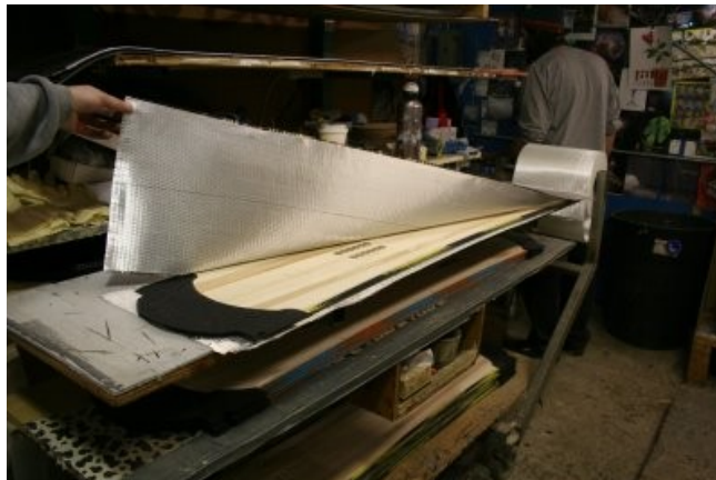
Figure 58: Fiberglass layer being placed on top of the wood core [26].
