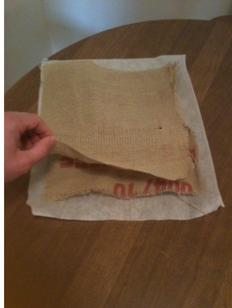
Figure 14: Creation of a laminate.
