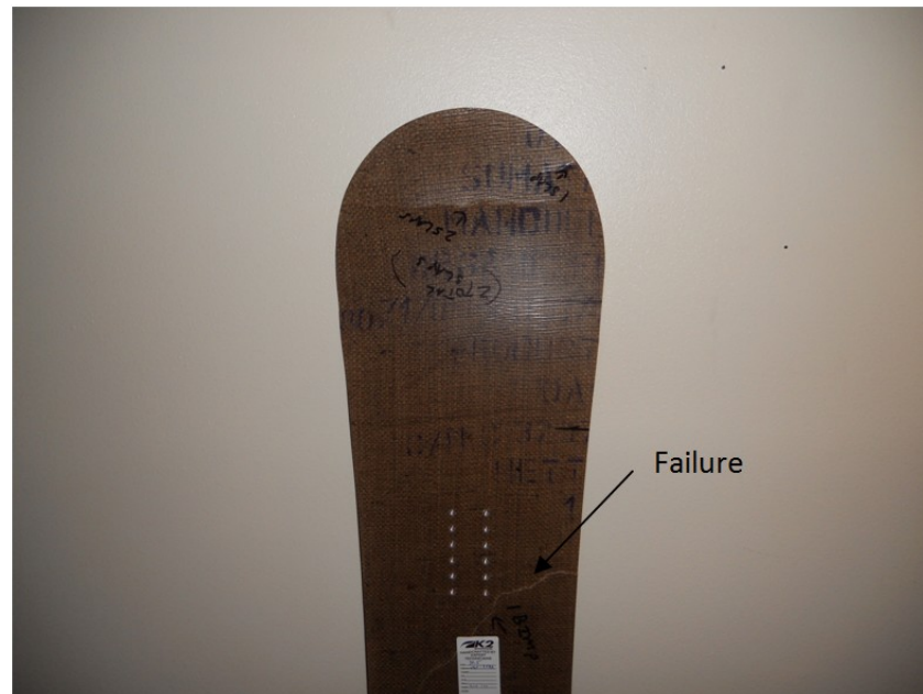
Figure 69: Terrain park impact failure.
