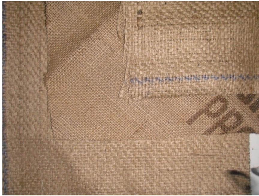
Figure 15: Layup 1 ( 0^{\circ}_B, 45^{\circ}_A, 0^{\circ}_B ).
