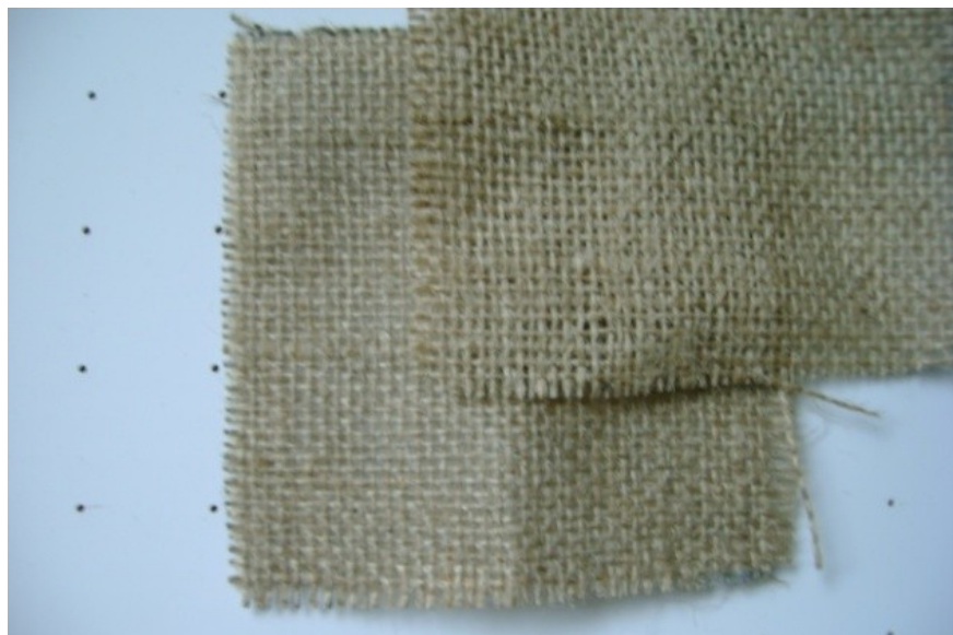
Figure 23: Layup 5 ( 0^{\circ}_A, 0^{\circ}_A ).
