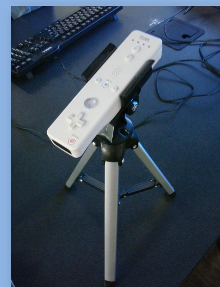
Figure 2 (left) – WiiMote stationed on stand (camera facing user) with adjustable viewing angle
