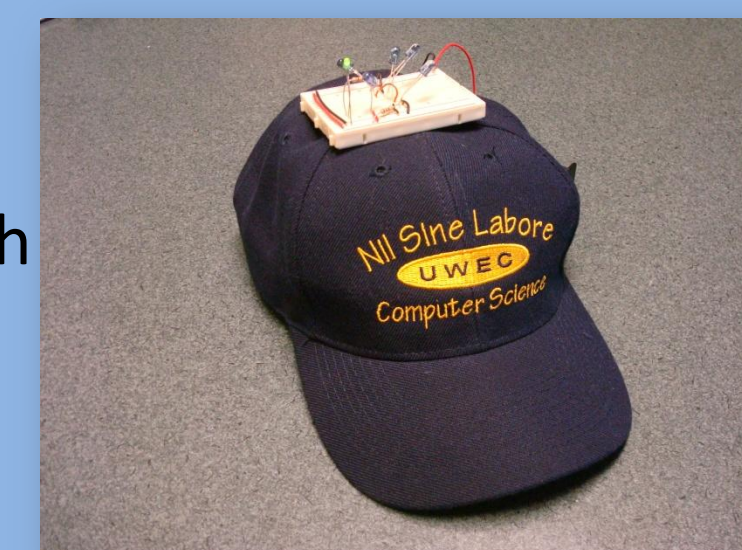
Figure 3 (right) – Hat outfitted with LED light cluster for WiiMote's camera viewing
