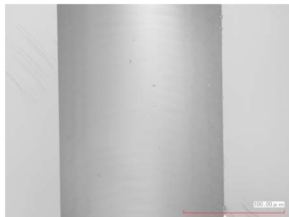
Fig. 2: Surface machined by carbide ball endmill
