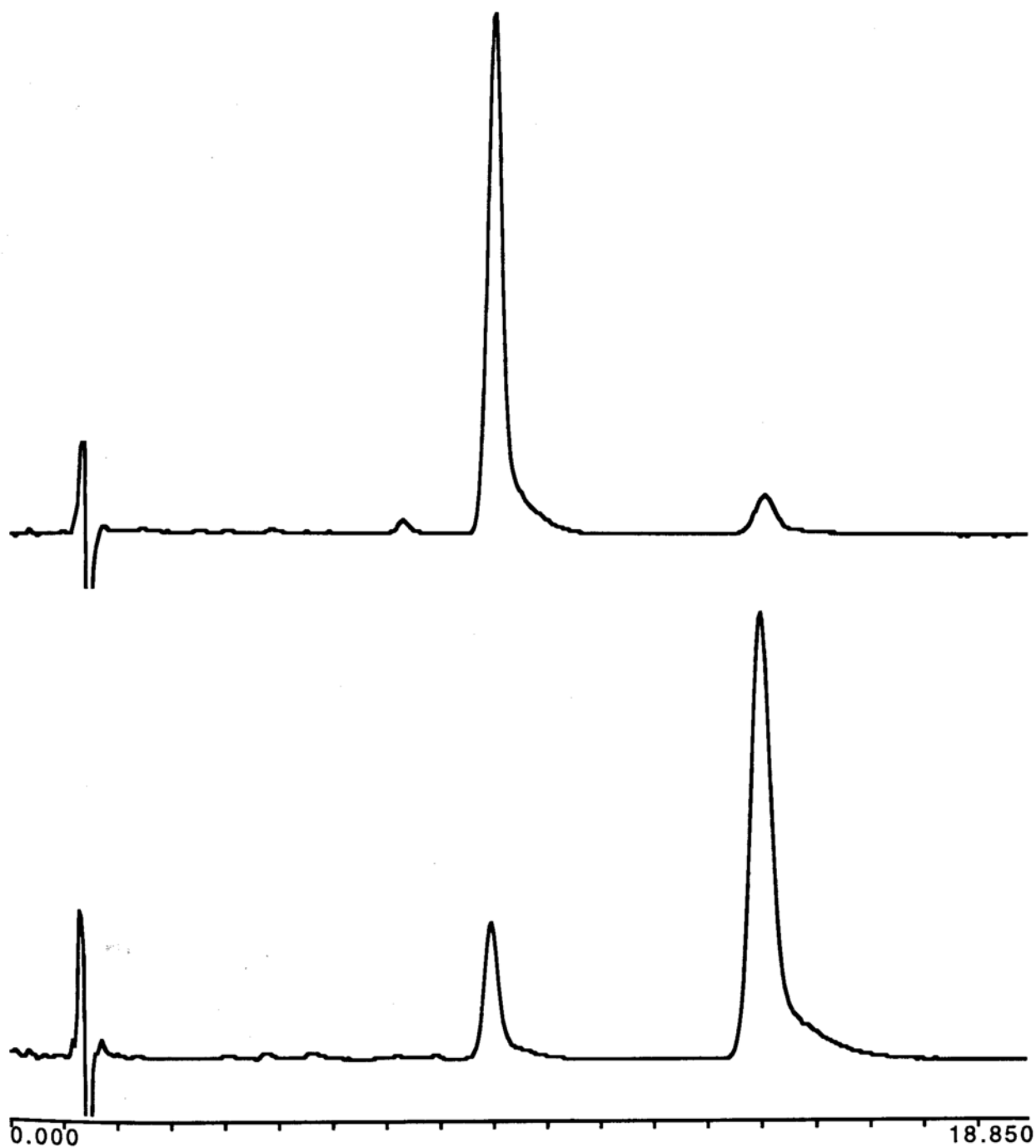
Figure IV-3 Typical HPLC chromatograms. Top : Drug stored in 0.4 M pH 8 buffer (with EDTA.2Na) after 10 days at 93°C, oxygen-purged, 91.1% A retained. Bottom : Drug stored in 0.2 M pH 8 buffer (with EDTA.Na) after 150 days at 93°C, air headspace, 19.6% A retained.
