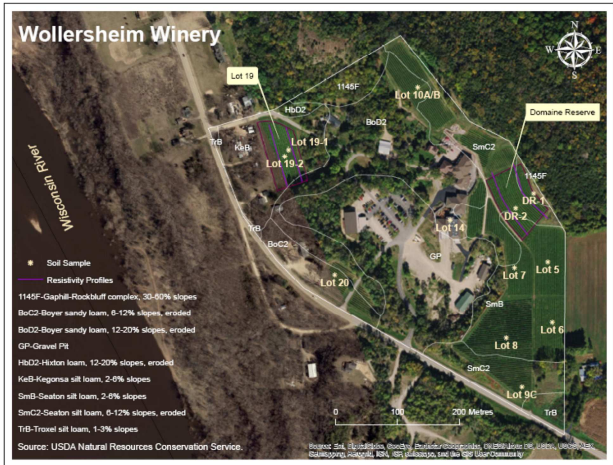
Figure 2-4. Location map of Wollersheim Winery vineyards illustrating the distribution of soil types, and soil sample and resistivity profile locations.
