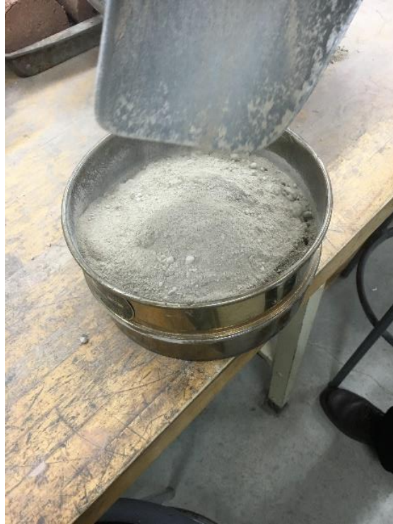
Figure 12 Photo shows soil in sieve#4
