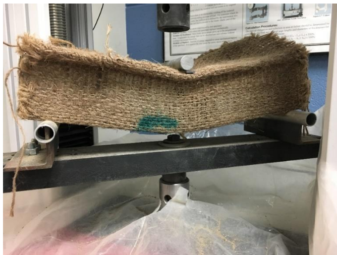
Figure 58 Failure shape of specimen wrapped and reinforced by burlap
