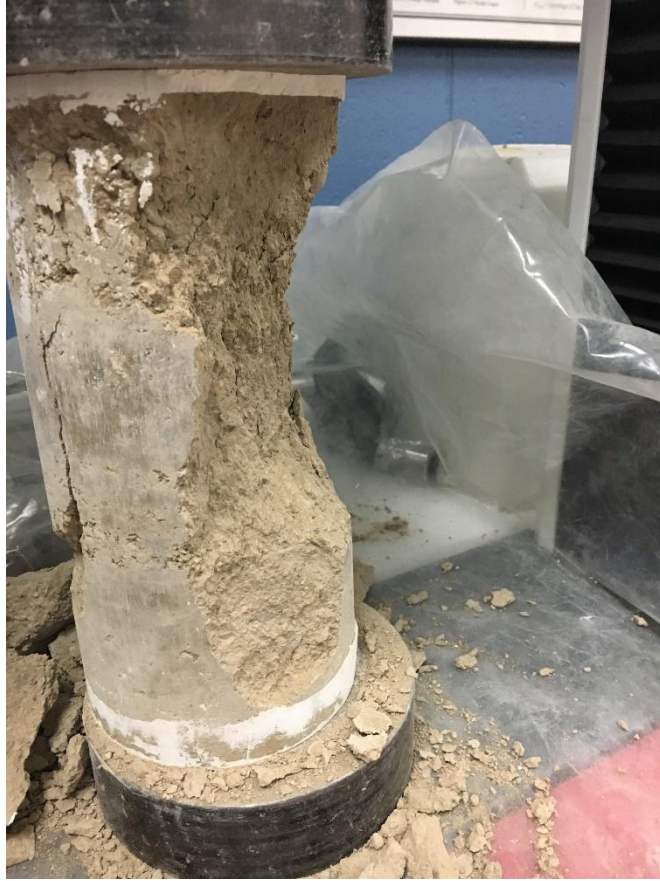
Figure 44 Shear failure of sample made of soil, 6% cement, and 6% fly ash C
