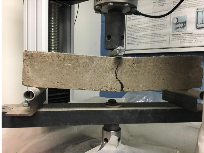
Figure 67 The final stage when the failure starts
