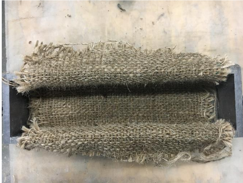
Figure 23 photo shows how to lay the first piece of burlap cloth
