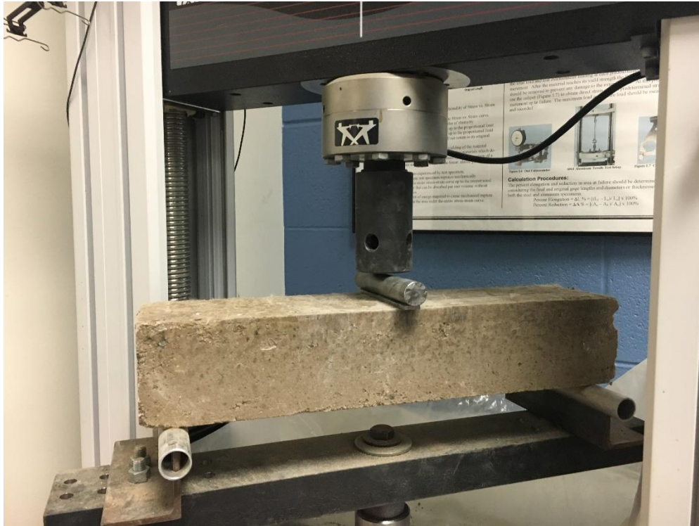
Figure 64 The specimen at the first, elastic, stage
