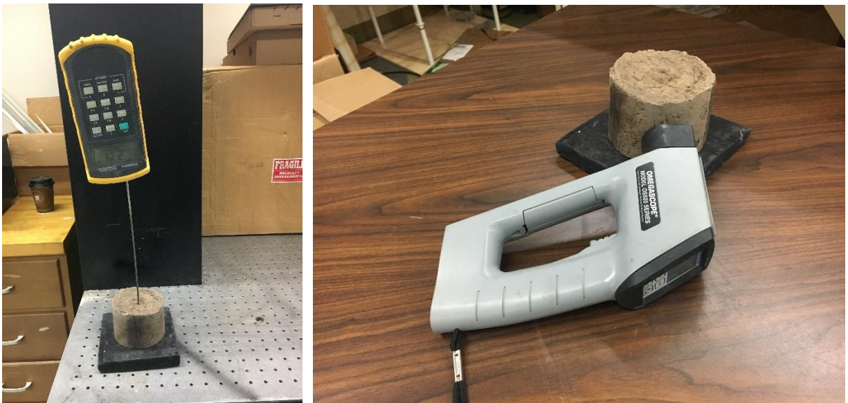
Figure 31 Pictures of portable digital thermometer (left) and handheld infrared thermometer (right)
