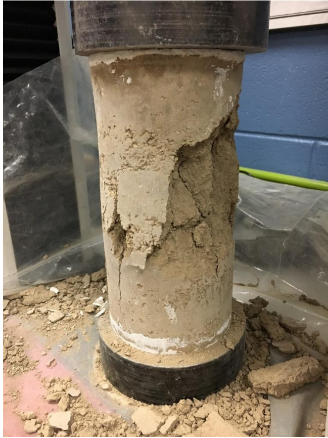
Figure 41 Shear failure of soil with 12% fly ash C
