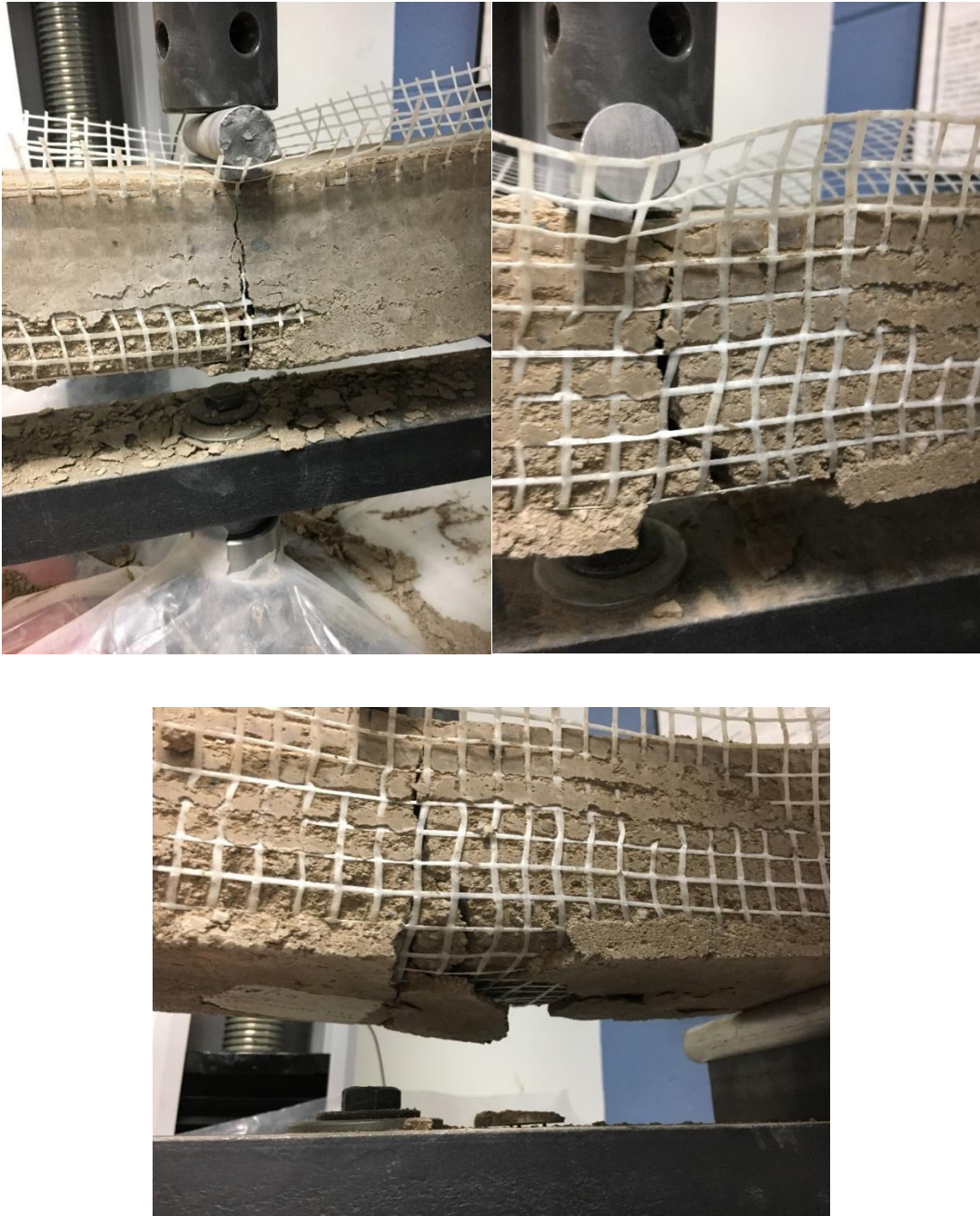
Figure 55 Pictures of beam reinforced by fiber mesh at failure
