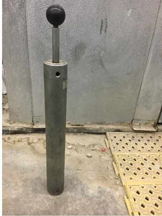
Figure 14 Hummer used to provide compaction energy
