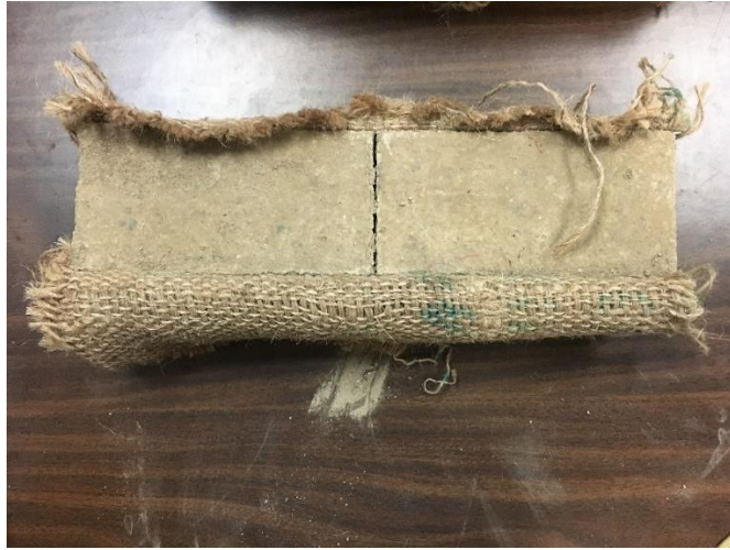
Figure 59 Crack at the maximum load
