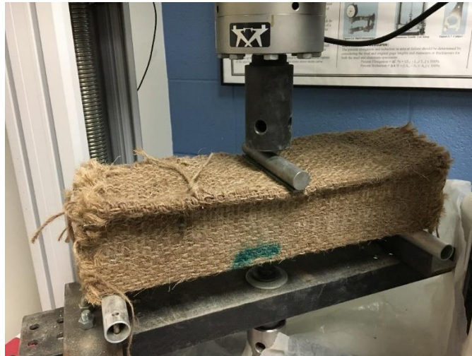
Figure 57 Loading of specimen wrapped and reinforced by burlap
