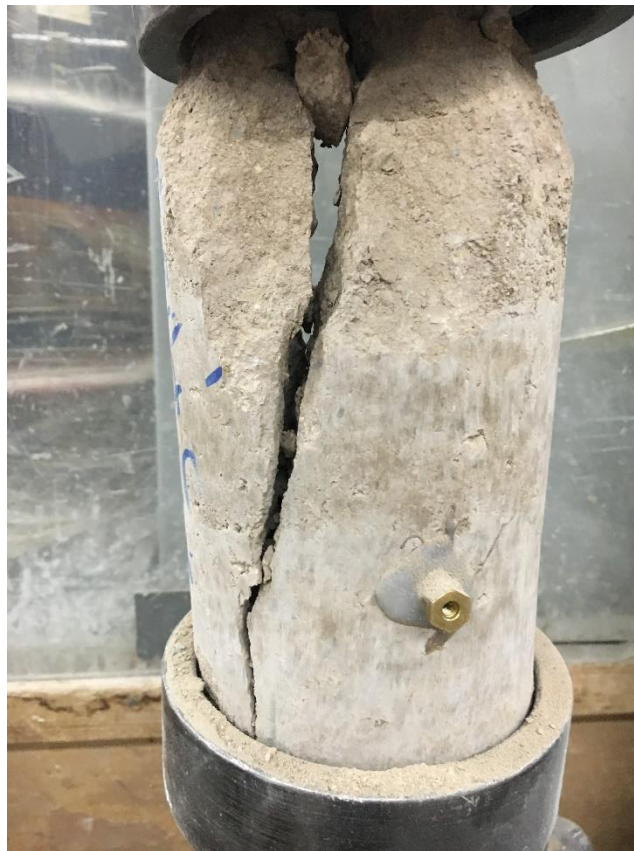
Figure 46 failure crack of a sample made of soil and 12% cement
