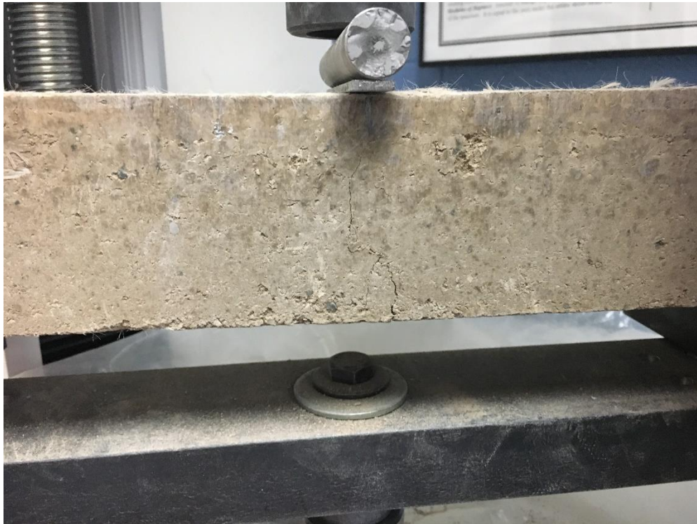
Figure 65 The second stage when the crack initiates
