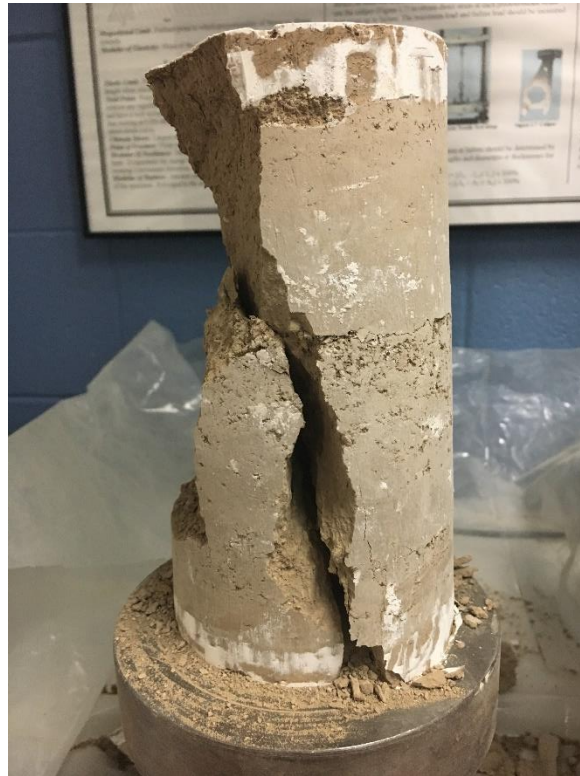
Figure 35 Photo of the specimen after fracture
