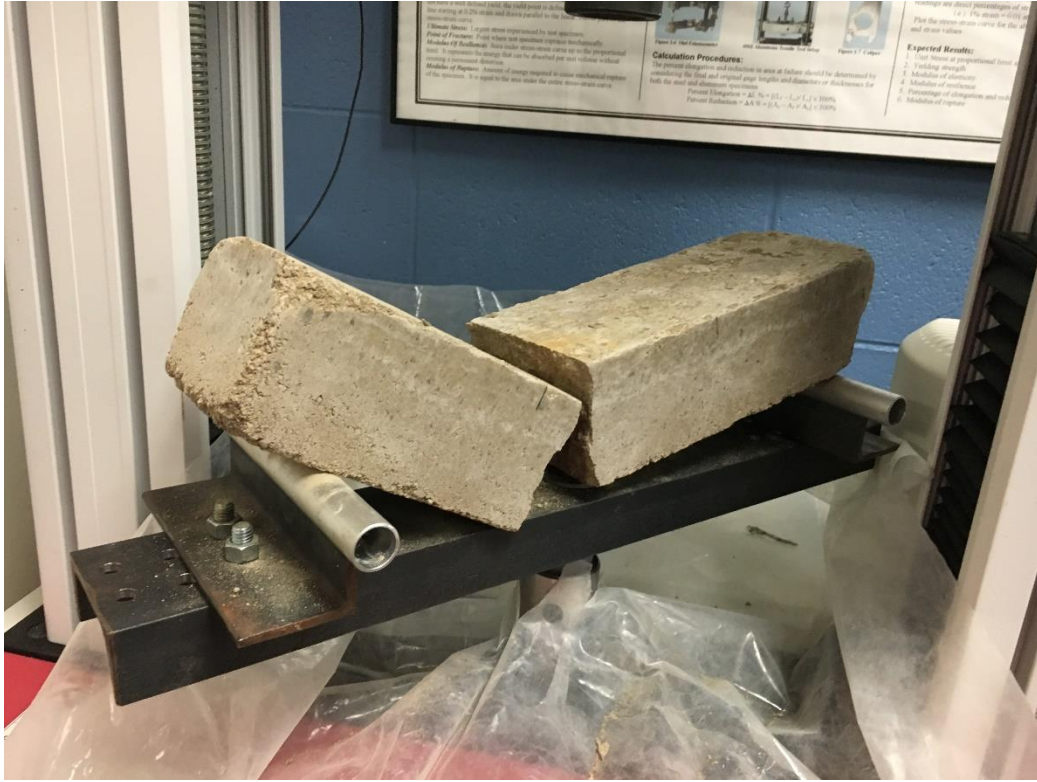
Figure 51 Tension fracture of a beam made of soil with 12% cement
