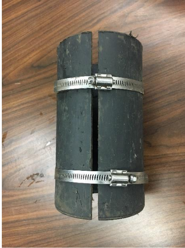
Figure 13 PVC mold used to prepare the cylinder sample
