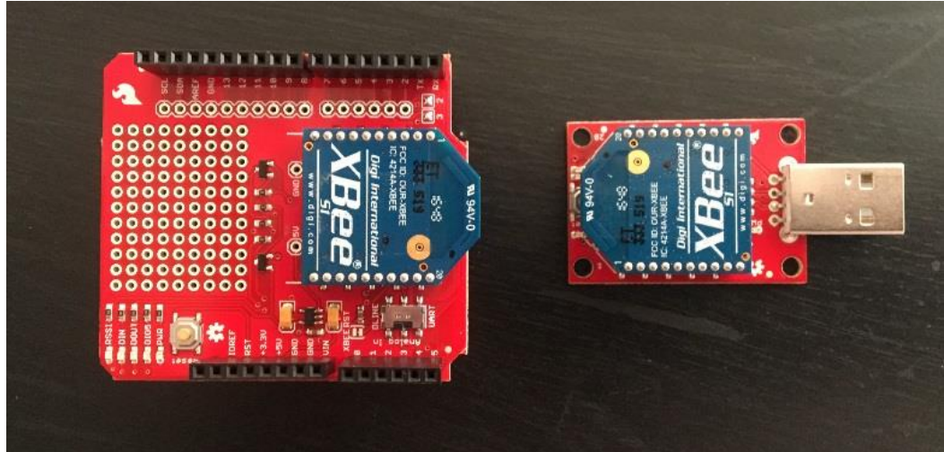
Figure 9: XBee S1 modules with Sparkfun Arduino Shield (Left) and USB Adapter (Right)
