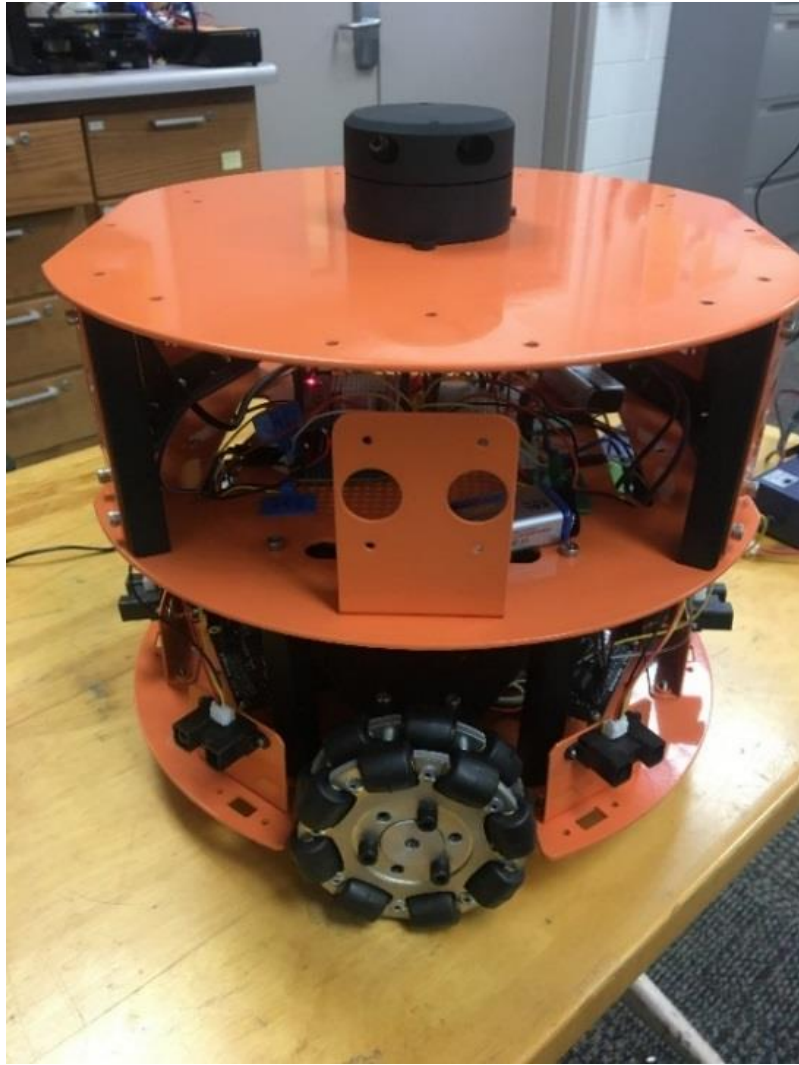
Figure 7: HCR Omni wheeled robot with LIDAR
