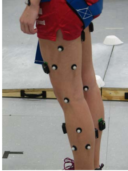
Figure 6: Picture of the motion capture sensors on the lower extremities.
