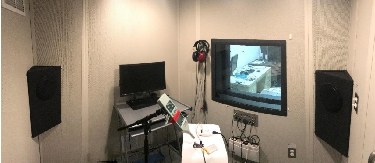
Figure 5-1 Hearing aids system testing setup in the sound booth
