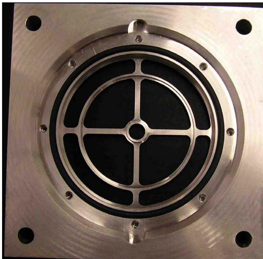
Figure 3.6. Backside of “cross hair” housing. This housing mates with the injector holder in Figure 3.5 to align and secure the injector and porous metal.
