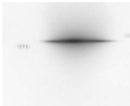
Figure 4.8. Overhead view of laser sheet scattered by fuel spray.
