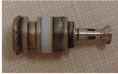
Figure 5.3. Inner structure of air-assisted injector. Two of the four holes are visible.
