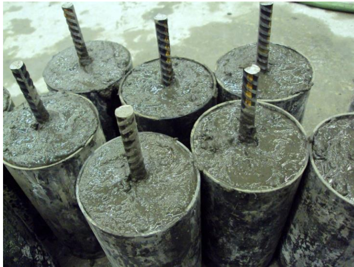
Figure 3.17: Cylindrical specimens for pullout test.
