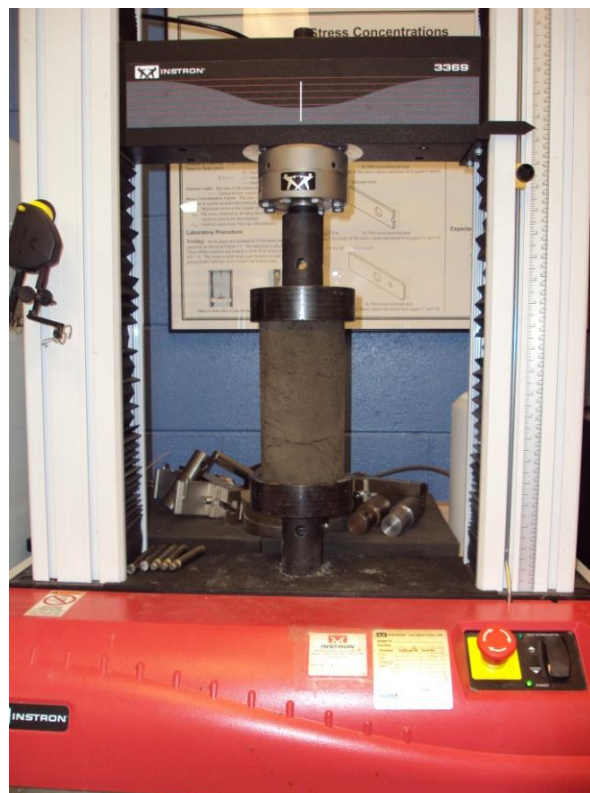
Figure 3.9: Compressive strength test setup.
