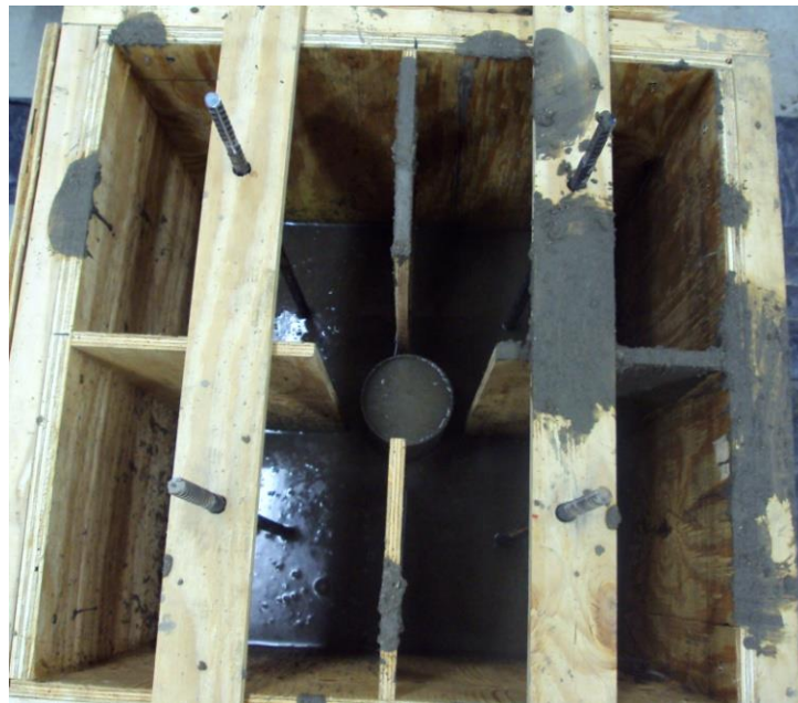
Figure 3.27: Cylindrical molds placed in the center of the box.
