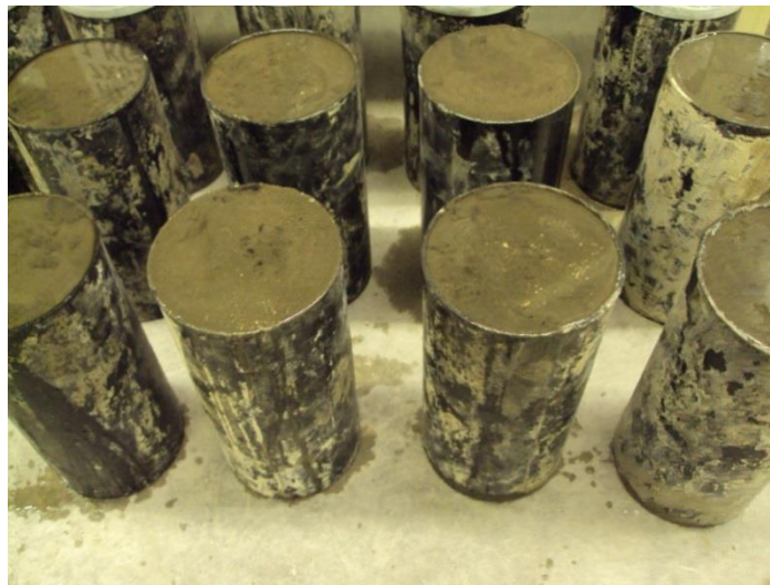
Figure 3.7: Cylindrical CLSM samples.
