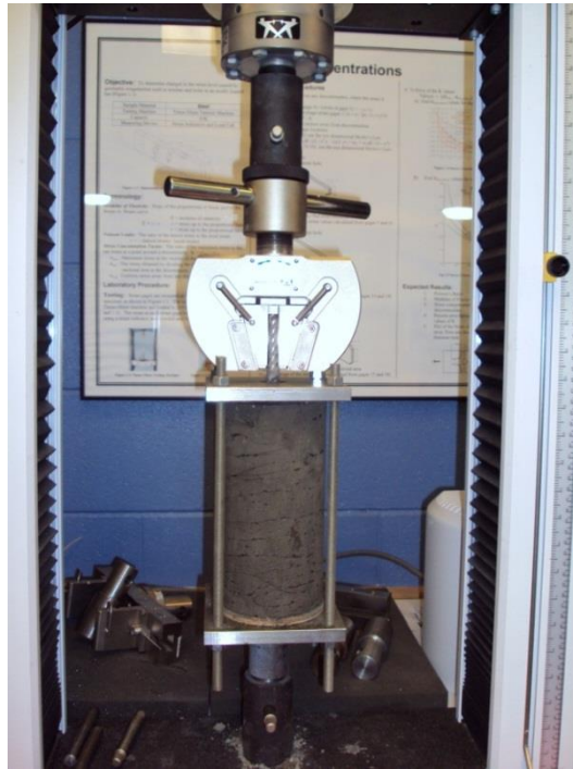
Figure 3.19: Pullout test setup on cylindrical specimens.
