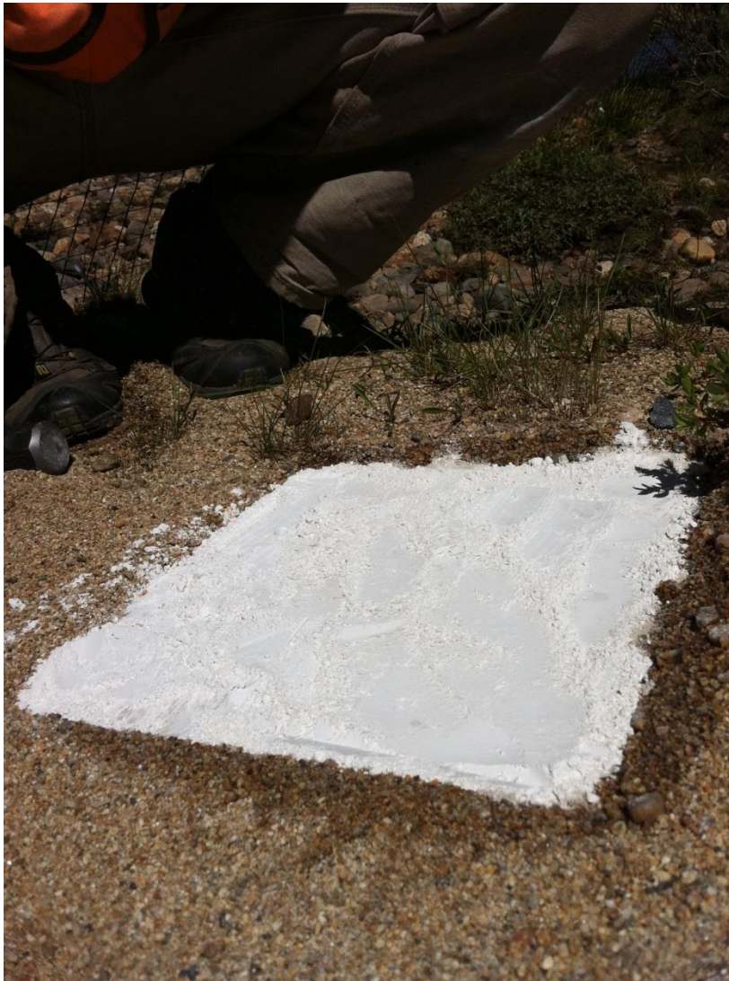
Figure 5: A completed clay pad receives a final addition of water to ensure it is completely moistened. Clay that is not moistened will easily be blown away in the wind.
