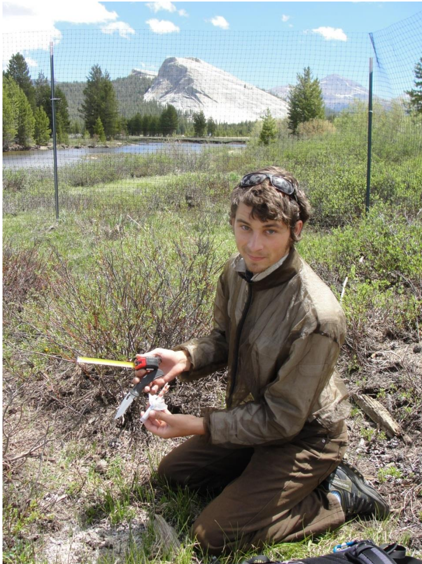
Figure 7: The materials required to take measurements from clay pads include: a tape measure, a coring device (plexiglass tube 15 mm in diameter and at least 4 cm long), a stick to push the sample core out of the coring device and back into the clay pad, a cloth to clean the sidewalls of the coring device, and a camera (not shown).
