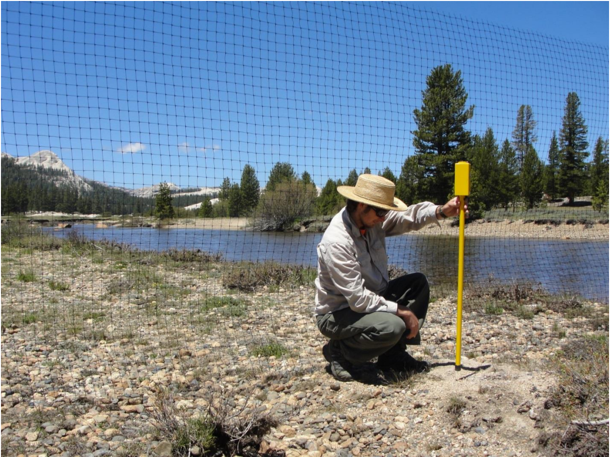
Figure 6: A clay pad buried in sand is located with a metal detector. Each pad can be located even if completely buried because the erosion chain installed in the middle of the downstream edge of the pad can be found with a metal detector.
