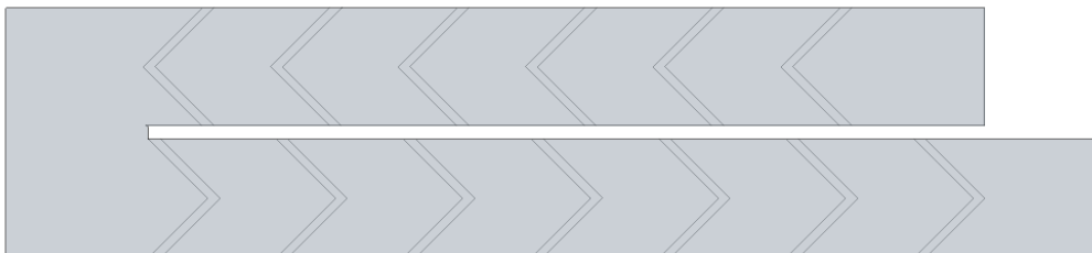
Figure 6-37: inlet/outlet for Channel with V-shape rib design two configuration P/e=10
