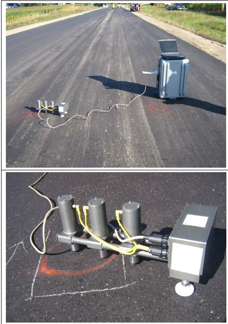
Figure 45. PSPA Being Used to Test the USH 45 HMA Overlay
