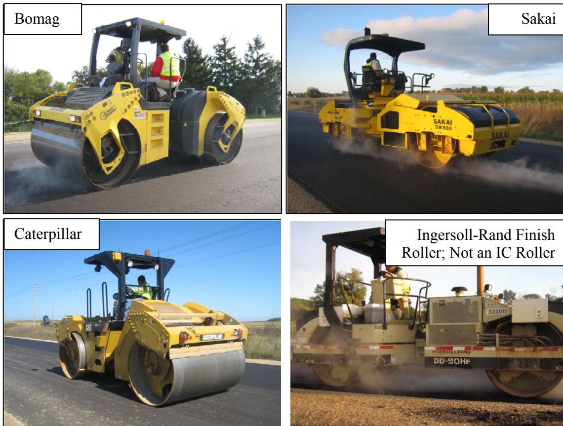
Figure 35. Eden USH 45 Project; IC and Other Rollers Used on the Project
