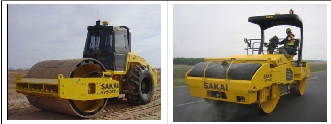
Figure 14. Sakai IC Rollers for Unbound Materials and HMA Mixtures
