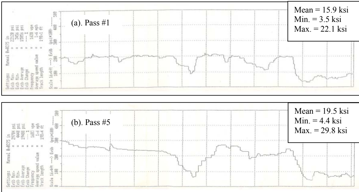
Figure 71. Charts from the Bomag IC Roller Showing the E_{vib} Values for Different Roller Passes; Jefferson Project; Crushed Aggregate Base, Right Lane, 2 nd Lift
