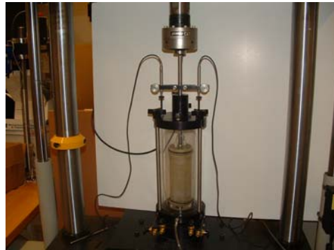
(c) Mounting the cell on the loading frame
