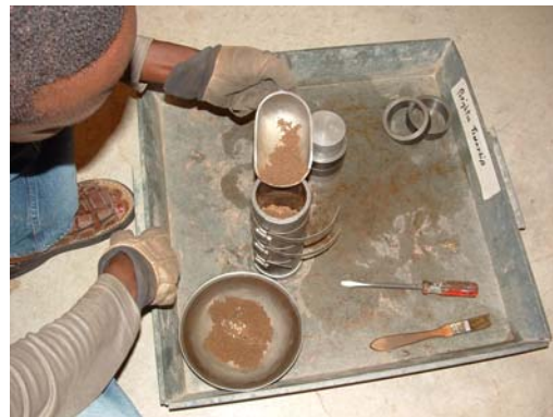
(b) Filling mold with one soil layer
