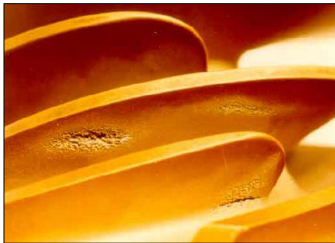
Figure 8: Localized cavitation damage on a pump blade [19]
