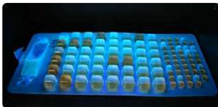
Figures 5, 6 (above) show Quanti-tray sealer as well as the Quanti-tray with both positive and negative results. Positive results show fluorescence.
