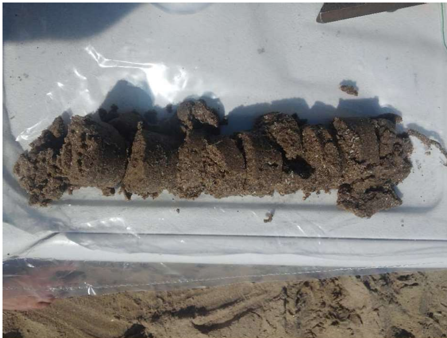
Figure 4 shows a typical core sample obtained in the field.
