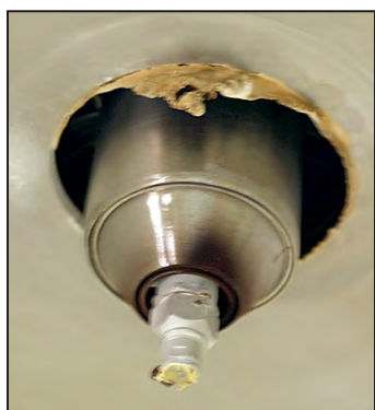
Spray dryer nozzle with burn on.
