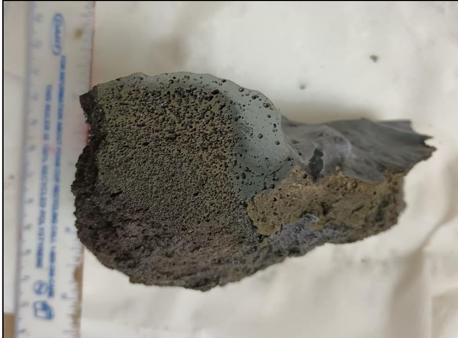
Figure 14 Photograph taken of sample KK_22_01 cross-section. Note the change in vesicularity between the outer surface and interior.
