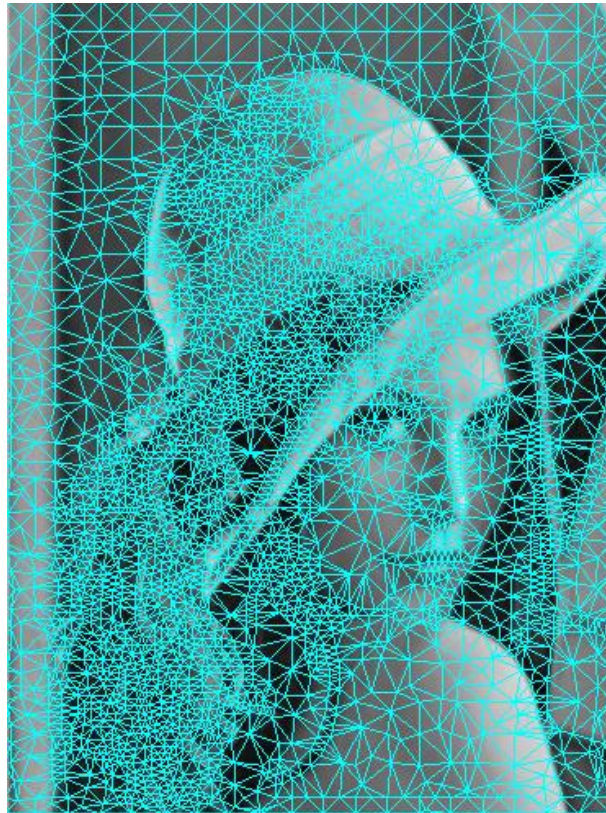
Fig 2.2: Initial triangle mesh generated by Delaunay triangulation.
