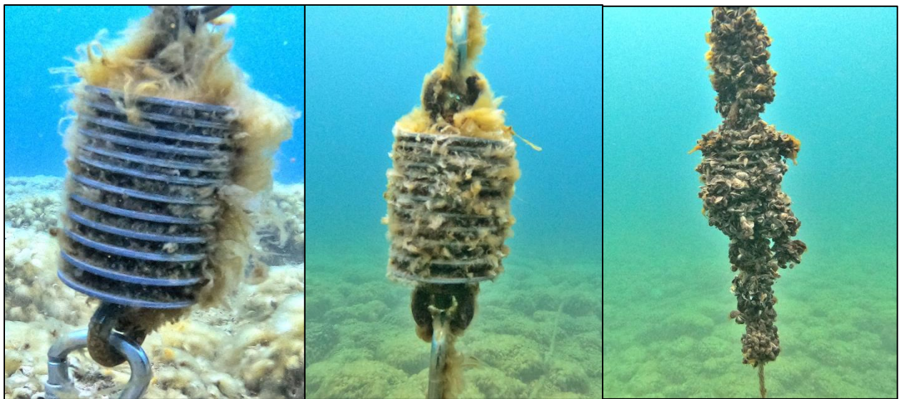
Figure 30. Hester Dendy traps populated with dreissenid mussels at SLBE. Bottom Hester Dendy trap (left) had mussels only growing between slots, 1-meter (middle) Hester Dendy had few mussels growing outside slots, and 2-meter (right) Hester Dendy trap had an abundance of dreissenid mussels growing inside and out of trap.
