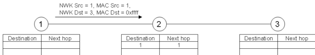
FIGURE 3.9: First Step in Routing
