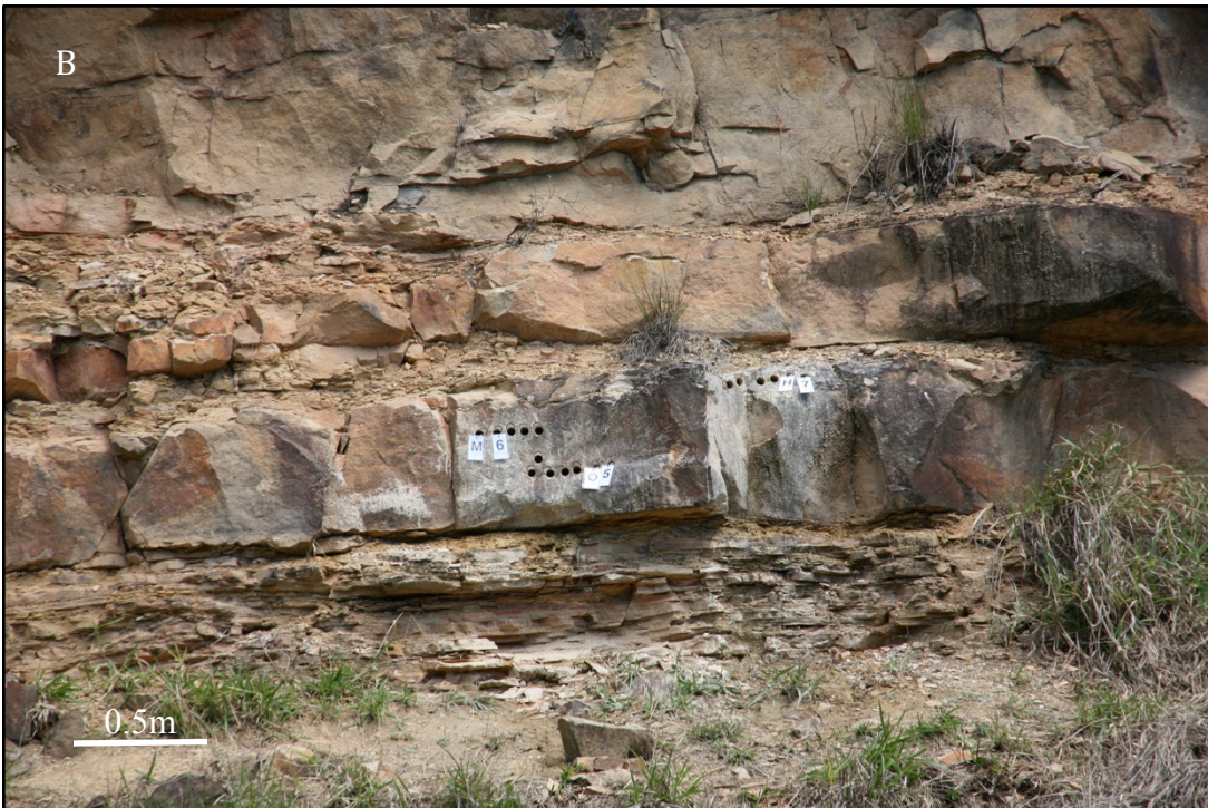
Fig 3-15. (A) Porto Amazonas road cut exposure located off Highway PR-427 in the state of Paraná. Yellow box indicates approximate location of (B) sample sites within a structureless sandstone (sites O5, M6, and H7).
