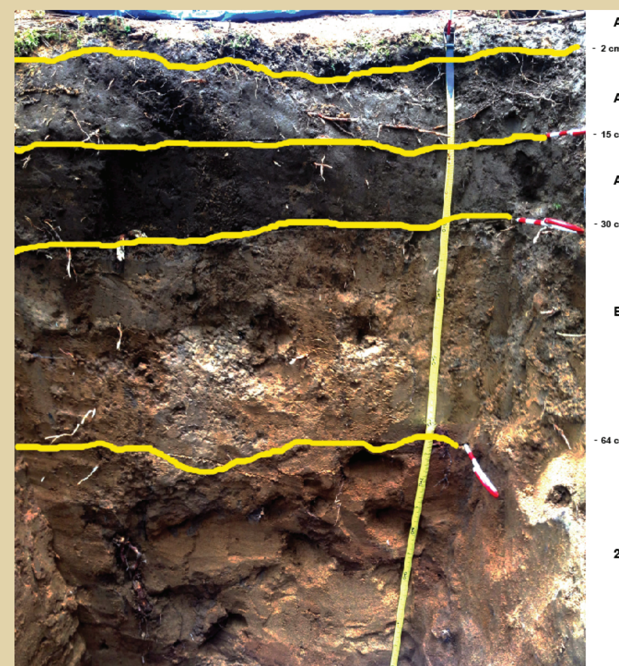
Figure 10. Photograph of soil profile 2014-3. Approximate horizon boundaries are shown by the yellow line. Horizon designations are on the right. This photo is a composite of two photos stitched at roughly 60 cm deep (Photograph by Matthew Brueske).
