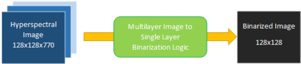
Figure 21: Schematic diagram of converting an HSI multilayer image into a binarized single layer image.
