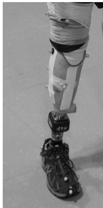
Figure 35: Prosthesis with iPecs sensor below the socket
