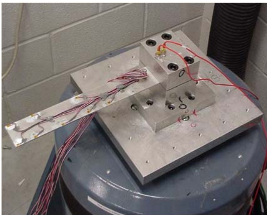
Figure 5.2 Clamped Cantilevered Beam Mounted on Shaker
