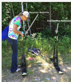
Figure 4. This GPR survey used a Sensors and Software pulseEKKO100 GPR system.
