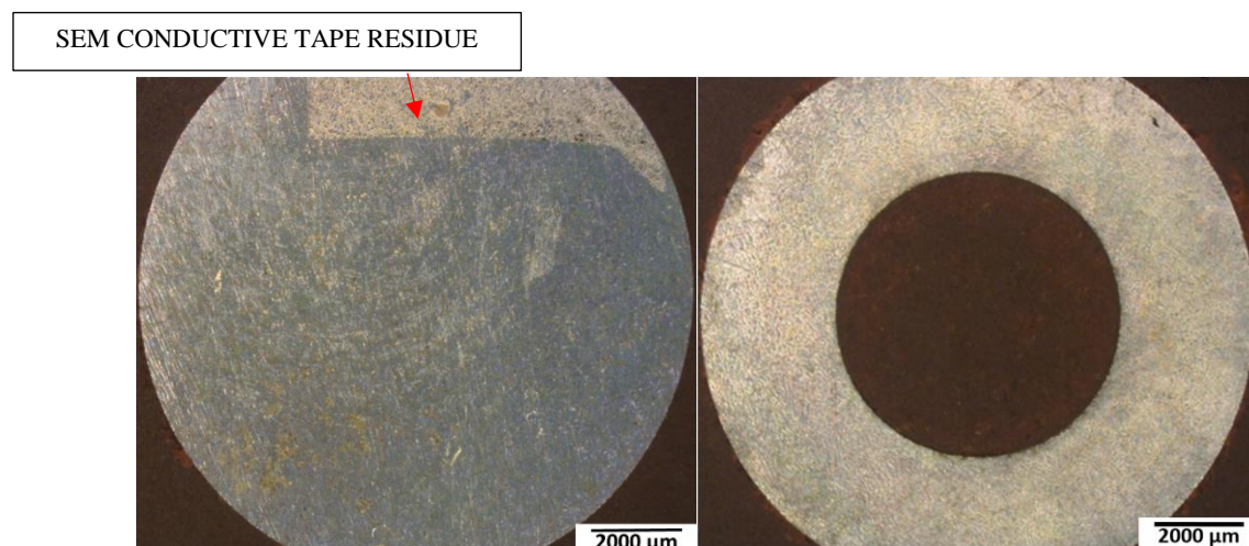
Figure 20: Cast magnesium (left) and cast magnesium machined tube (right) etched and seen under a Zeiss Stemi2000-C Stereomicroscope at 6.5x to see the general shape and structure of the material.
