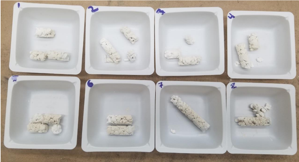
Figure 6: Large spacer material after heat treatment.
