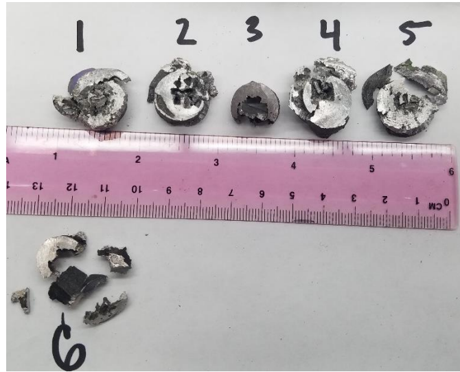
Figure 16: Compressed medium pore size samples
