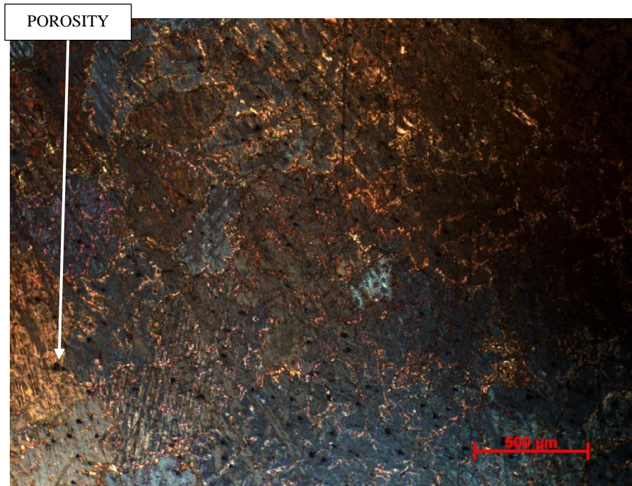
Figure 22: Magnesium stock ingot etched with 150mL ethanol, 50mL deionized water, and 1 mL glacier acetic acid at 50x taken with AX10-Zeiss Microscope under polarized light. This image is showing magnesium stock ingot metal after machining.
