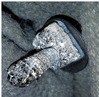
Figure 10: Condensed magnesium on chill system for infiltration process.
