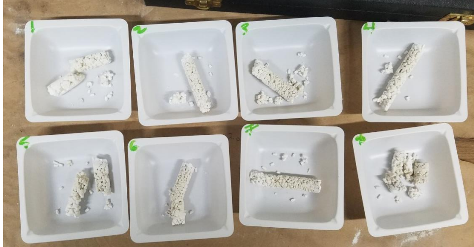
Figure 8: Small spacer material after heat treatment.
