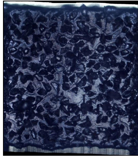
Fig. 3: Stitched Imaged Surface of 0.5mm OD, #120 Grit Diamond Grinding Wheel.
