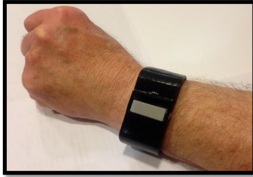
Figure 34: The final desired TheraBracelet device with batter, amplitude adjusting controlling, sound file, and battery all able to be housed on the wrist.
