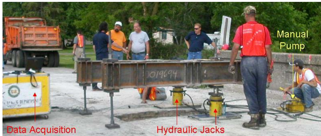
Figure 6.12. Preparing to execute load test on west section
