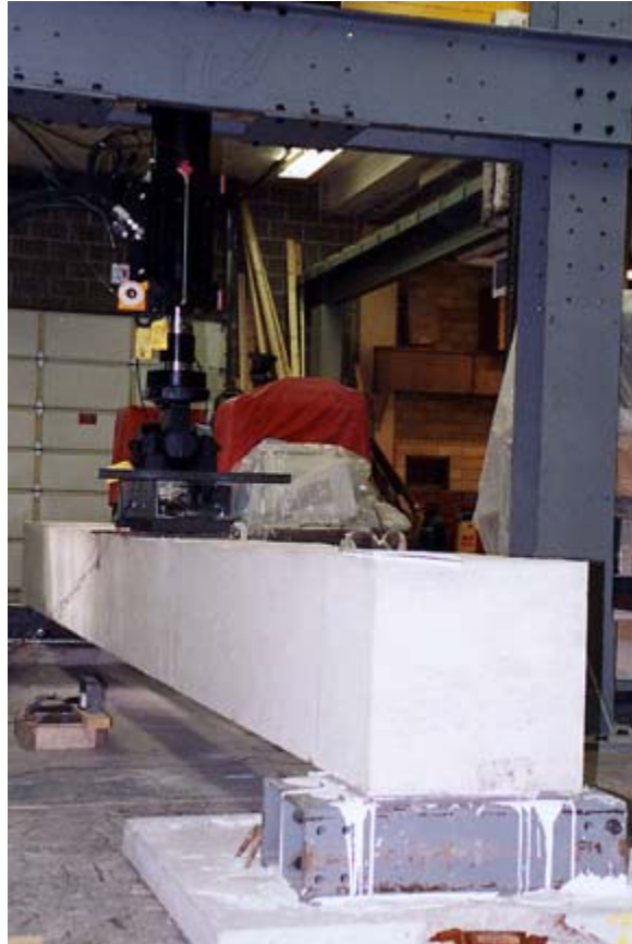
Figure 5.11. Laboratory beam in test frame
