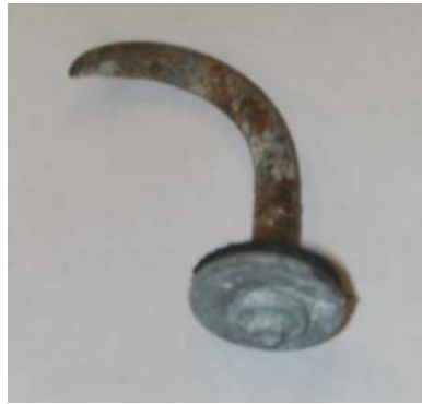
Figure 6.43. Corrosion on X-ALH fastener seen after ten months
