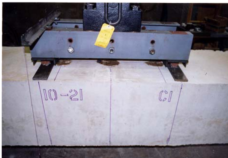
Figure 5.12. Close-up of spreader beam used for loading
