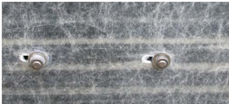
Figure 5.32. Bearing failure seen at fasteners in beam FRP 2SS
