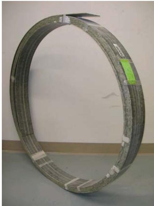
Figure 4.16. Roll of 100 ft long FRP strips as supplied by the manufacturer
