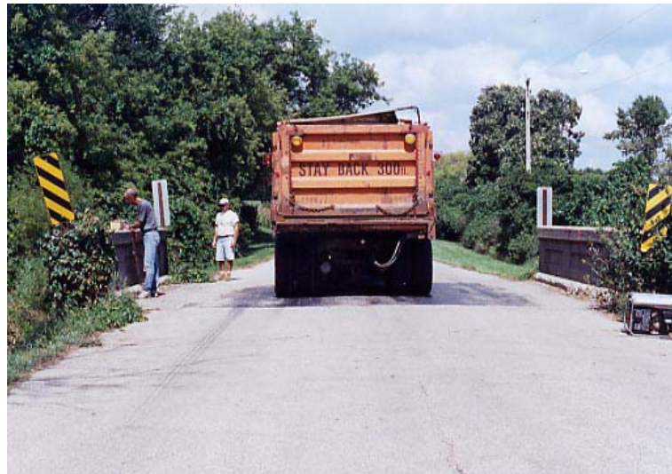
Figure 4.36. Load Case I on bridge P-53-702
