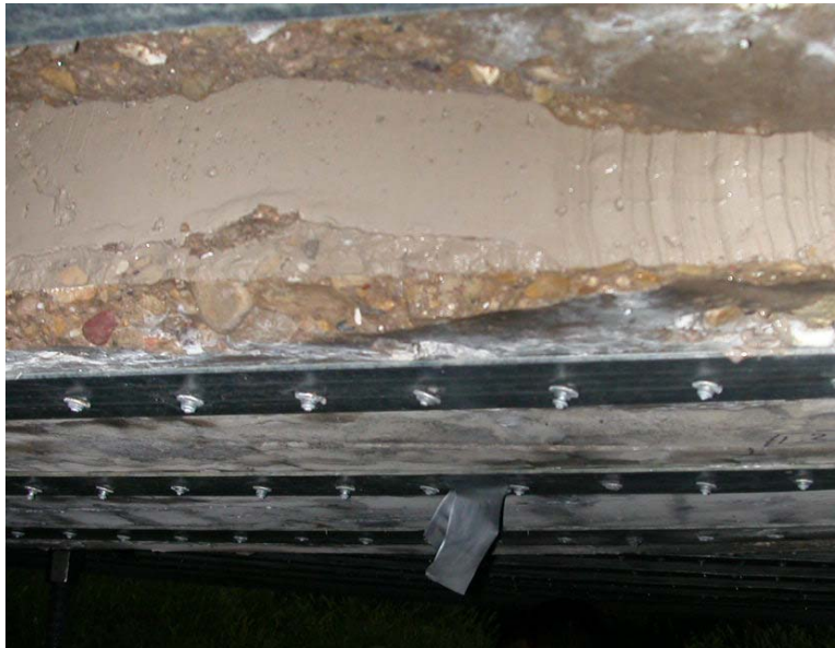
Figure 6.21. View of rotated fasteners along length of west section
