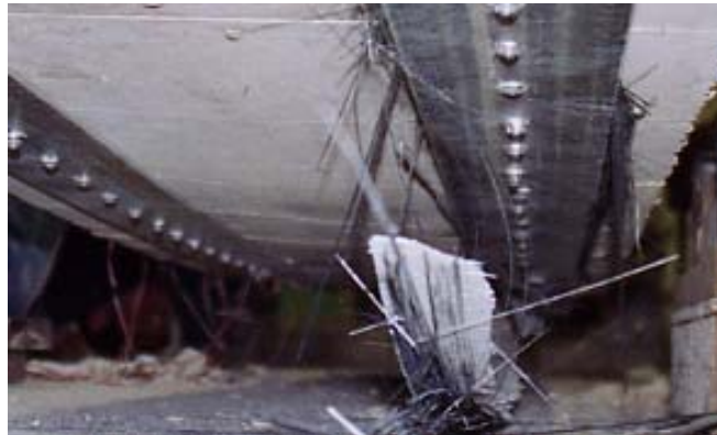
Figure 5.34. Rupture of FRP strip in beam FRP 2SS
