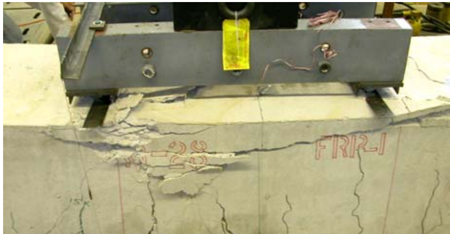
Figure 5.22. Concrete compression failure of FRP1
