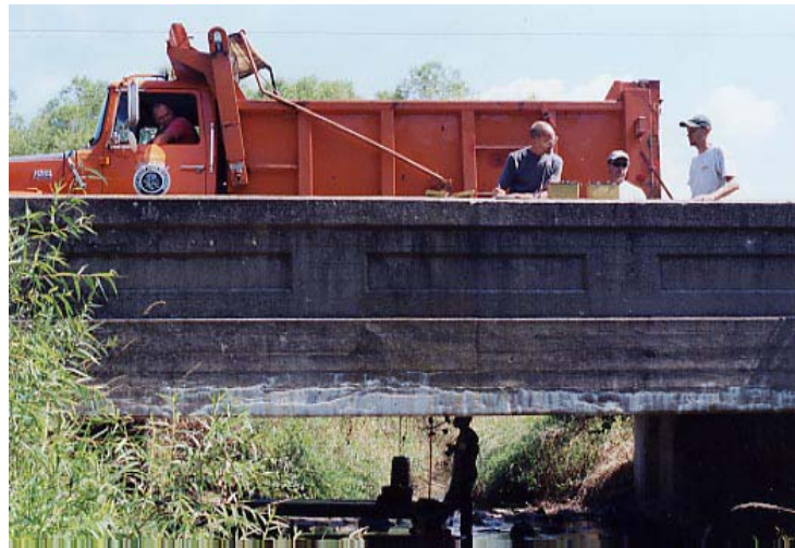
Figure 4.32. Service load tests on bridge P-53-702
