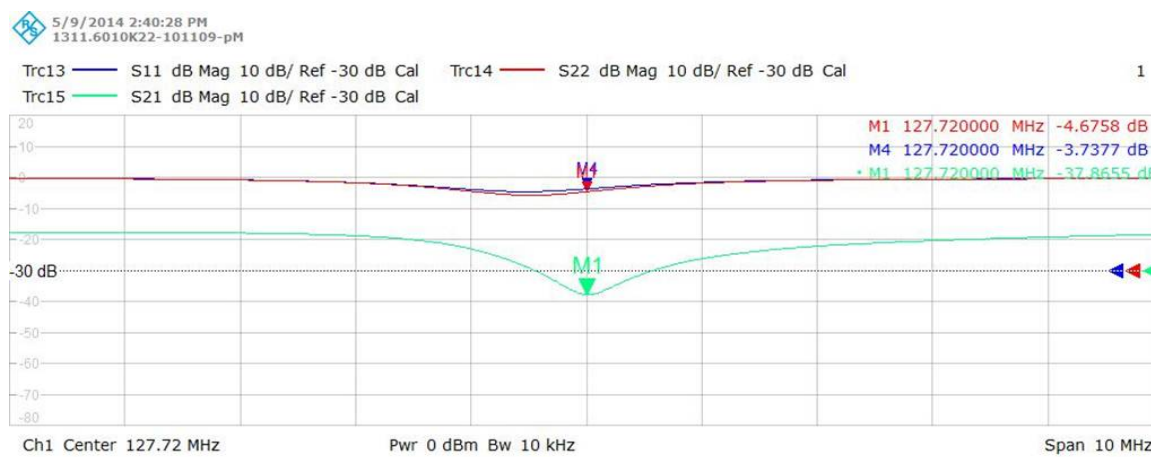
Figure 10: S-parameters measured on prototype body coil.
