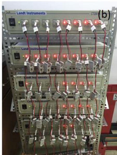
Figure 2.3(a) Hitachi H-9000NAR high resolution TEM, (b) Landt battery test system, (c) Gamry electrochemical workstation.
