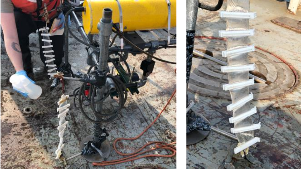
Figure 2.11 The membrane tube attached in the UWMPIV frame
