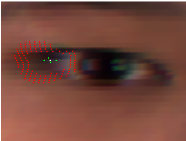
Figure 4.3: An example of selecting the positive (green and white (ground-truth)) and negative (red) class samples for the training dataset.
