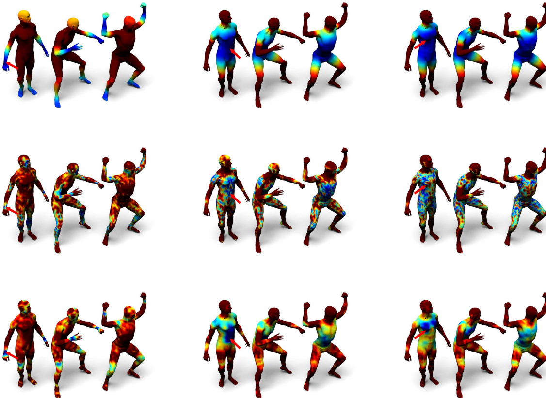
Figure 2.4: The comparison between HKS (first row), WKS (second row), and the data-driven spectral descriptors (third row) proposed in [5]. The Euclidean distances between the extracted descriptors for the white points (shown by red arrows) in each model were computed and visualized from the highest (red) to the lowest (blue). As it is observed, HKS finds the correspondence areas with high specificity, however, it is not sensitive enough. In fact, the areas illustrated with the blue color are connected but they are too large. On the other hand, the blue area in WKS are smaller, however, they are spread all over the model. The proposed descriptors in [5], enjoy both advantages to some extent. As it is observed, the blue areas in the third row, are smaller than the ones obtained using HKS. Besides, they are denser compared with those of WKS. This figure is taken from [5].
