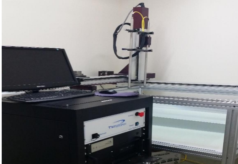
Figure 4.1: TecScan Computer Controlled Ultrasonic Immersion tank
