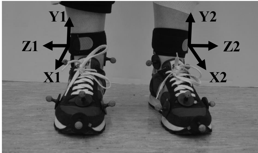
Figure 15. Orientation of the axes for each accelerometer.
