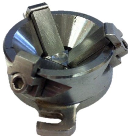
Figure 20 Anton Paar tribology measuring cell – photograph of holder for base plates. The holder in the photograph has metal surface plates installed in the three holding spots. The metal plates can be easily replaced with Teflon plates using Allen wrench.
