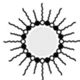
Figure 14 Illustration of surfactants forming physisorbed layer around a particle (Biresaw 2009).
