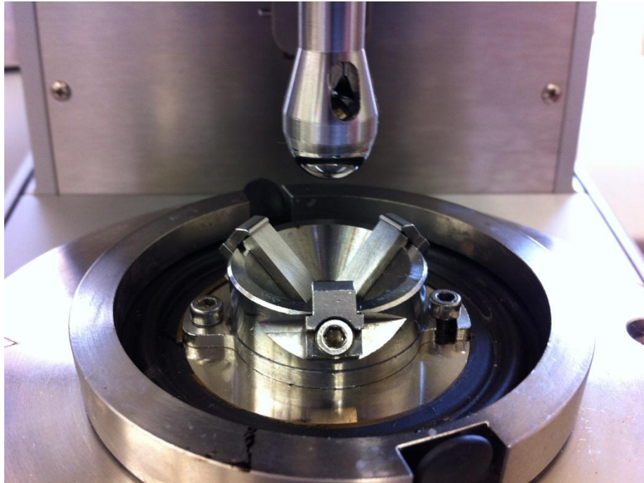
Figure 19 Anton Paar tribology measuring cell – photograph of chromed steel ball attached to measuring system shaft and holder for base plates. The whole assembly is ready for sample placement.
