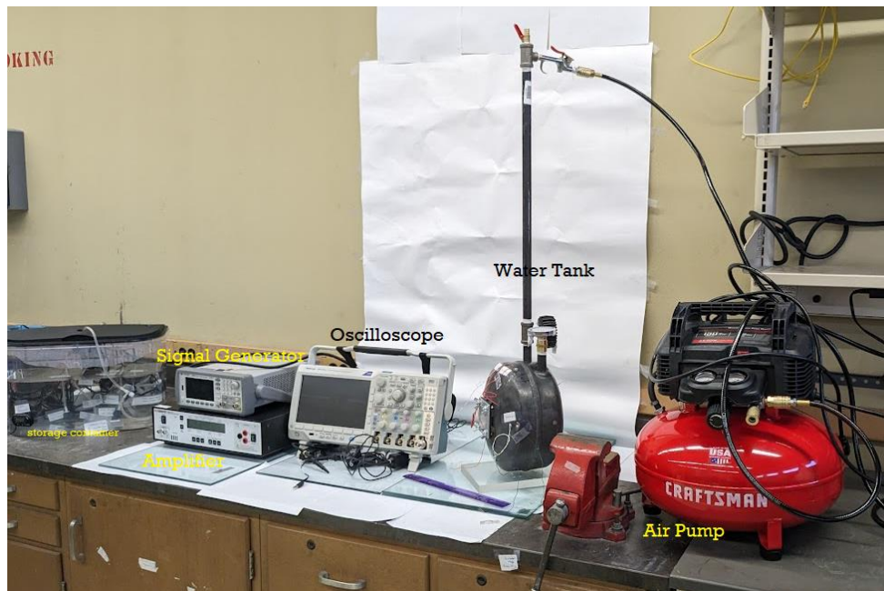
Figure 5. 9: Experimental setup for the pressure vessel
