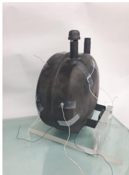
Figure 3. 1: Water tank mounted on support with PZTs attached.
