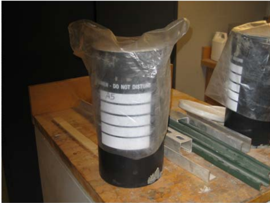
Figure 6.1 Cylinder in Mold with Plastic Cover.
