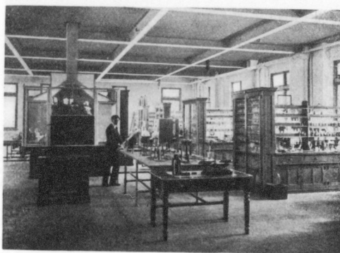
Analytical and Experimental Department: To the right may be seen a number of "working sections," each 14x15 feet in extent and separated from one another by low partitions—a plan that affords the necessary isolation for individual work and yet does not interfere with lighting, heating, and ventilation. In the foreground is a large work-table of iron with alborinestone top. This table, as well as those in the working sections, is fitted with hot and cold water supply, steam, compressed air, mechanical vacuum, gas, and water at high pressure for use with the aspirator pump. To the left may be seen a large hood of glass and iron, fitted with steam and sand baths, with special provision for ventilation.
