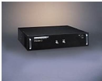
FIGURE 3.2: The Precision LC tester [2]. Not shown is the external testing bay that connects to the drive and return ports on the front of the tester.
