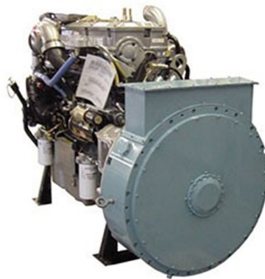
Figure 4. PA57-1000 Single Rotor, Dual Stator PM 1000hp Generator [40]
