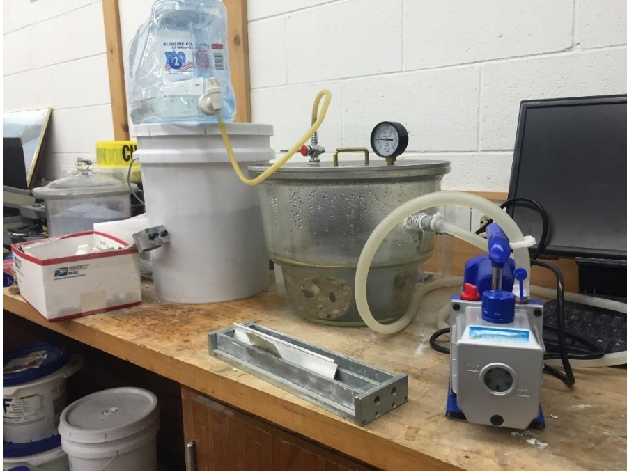
Figure 3.6: Concrete samples covered by de-aerated water in a vacuum desiccator.
