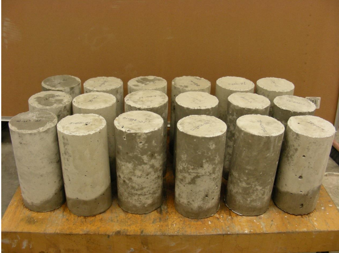
Figure 3.1: The cylinders were subjected to freeze-thaw cycles or combination of freeze-thaw cycles and compressive stress.
