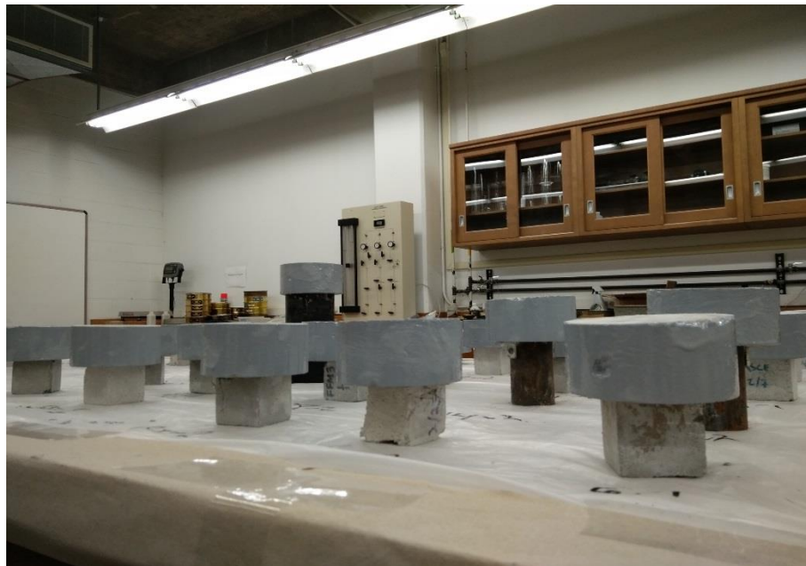
(b)Specimens after coating
