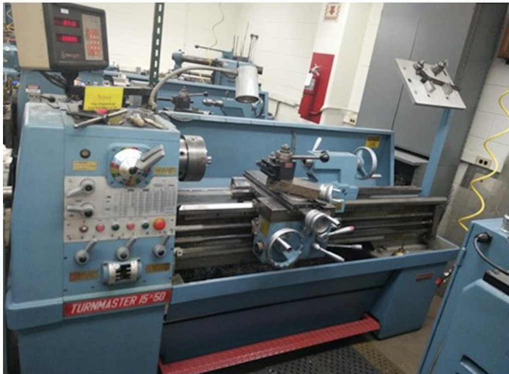
Figure 3.5: Milling sample surfaces using AMERICA TURNMASTER 1525 Engine Lathe
