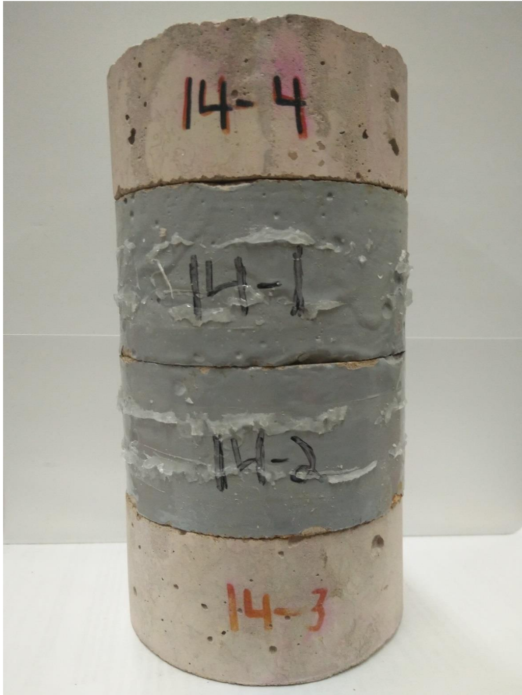
Figure 3.2: The samples for RCIP tests are from middle of cylinders.
