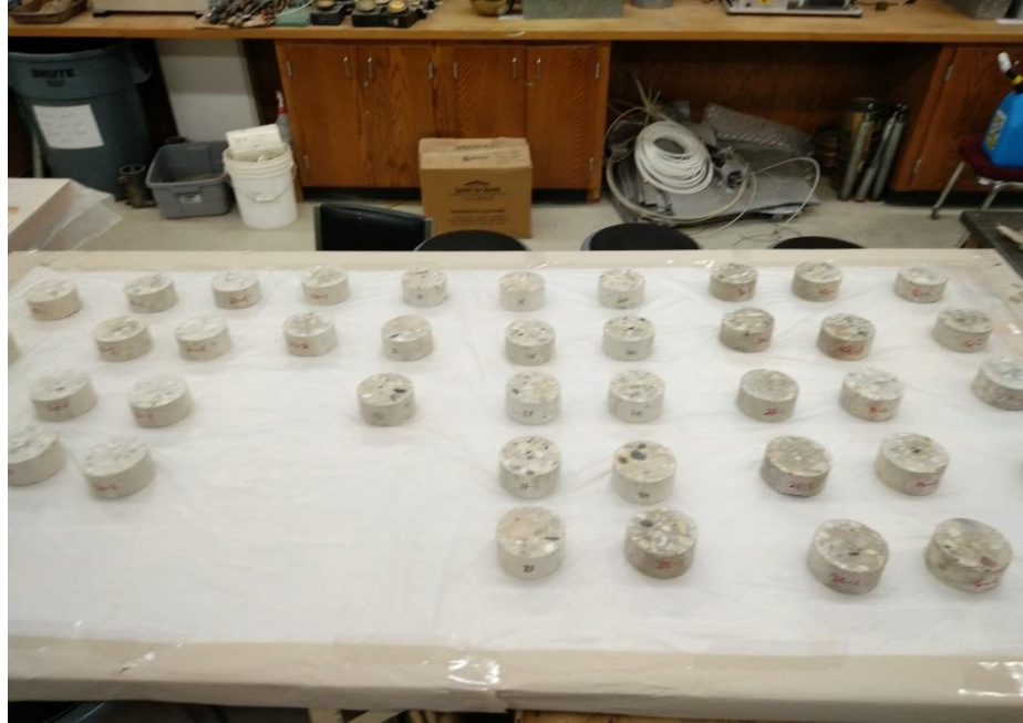
(a)Specimens before coating
