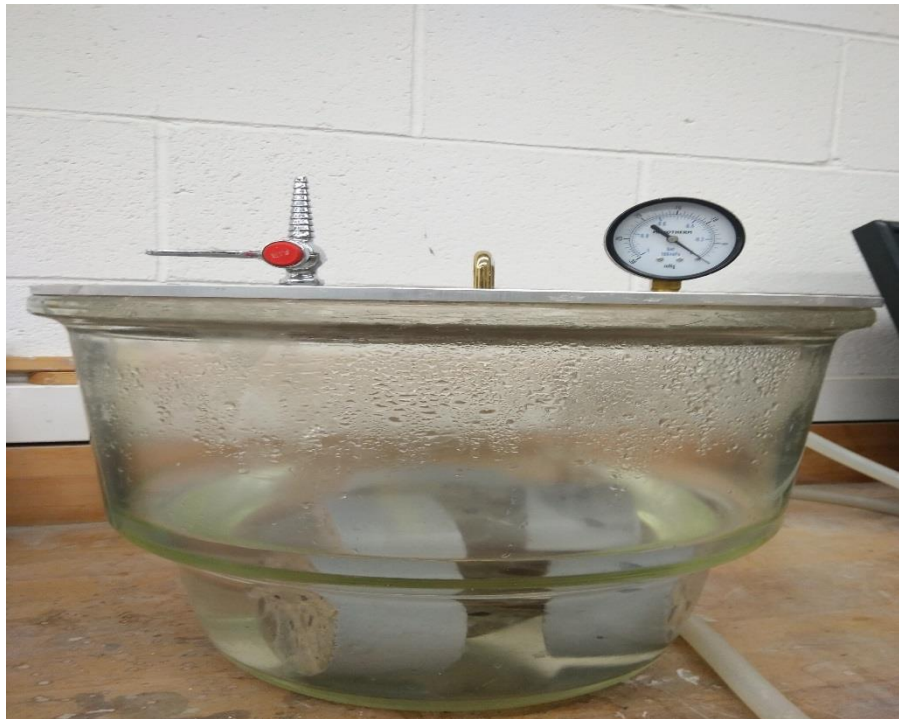
Figure 3.7: test specimens immersed in de-aerated water under atmospheric pressure.
