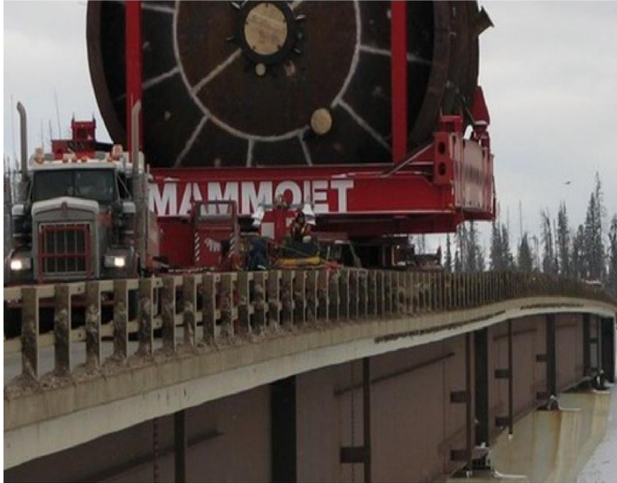
Figure 1.1: Overweight vehicle causing visible deflection in bridge (Lin et al., 2012)
