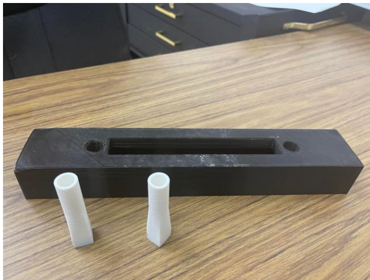
Figure 3-4: Air and water inlet manifolds 3-D printed parts
