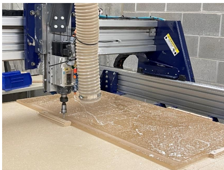
Figure 3-2: Machining the set-up covers using UWM CNC machine
