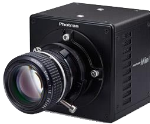
Figure 3-8: Photron Fastcam Mini UX high-speed camera
