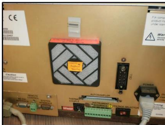
Figure 1. Photograph showing the location of the air filter on the back of the FIMS-100 Mercury Analyzer.
