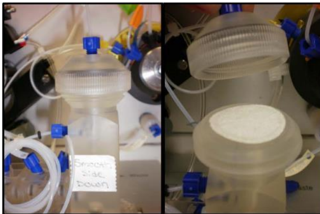
Figure 7A and 7B. Photograph showing the gas/liquid separator and the filter in placement in the gas/liquid separator.
