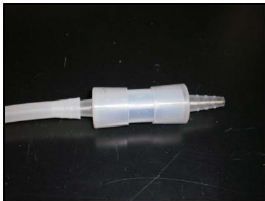
Figure 2. Photograph showing the mercury filter attached to the silicon tube.
