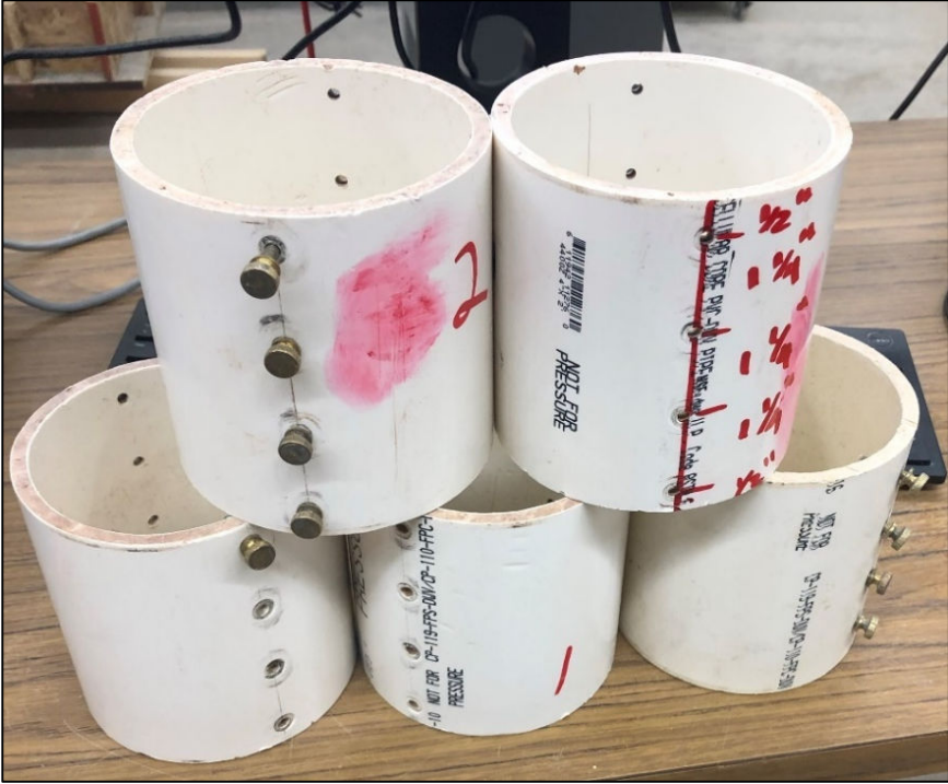
a) Four holes on each side for the plastic mold
