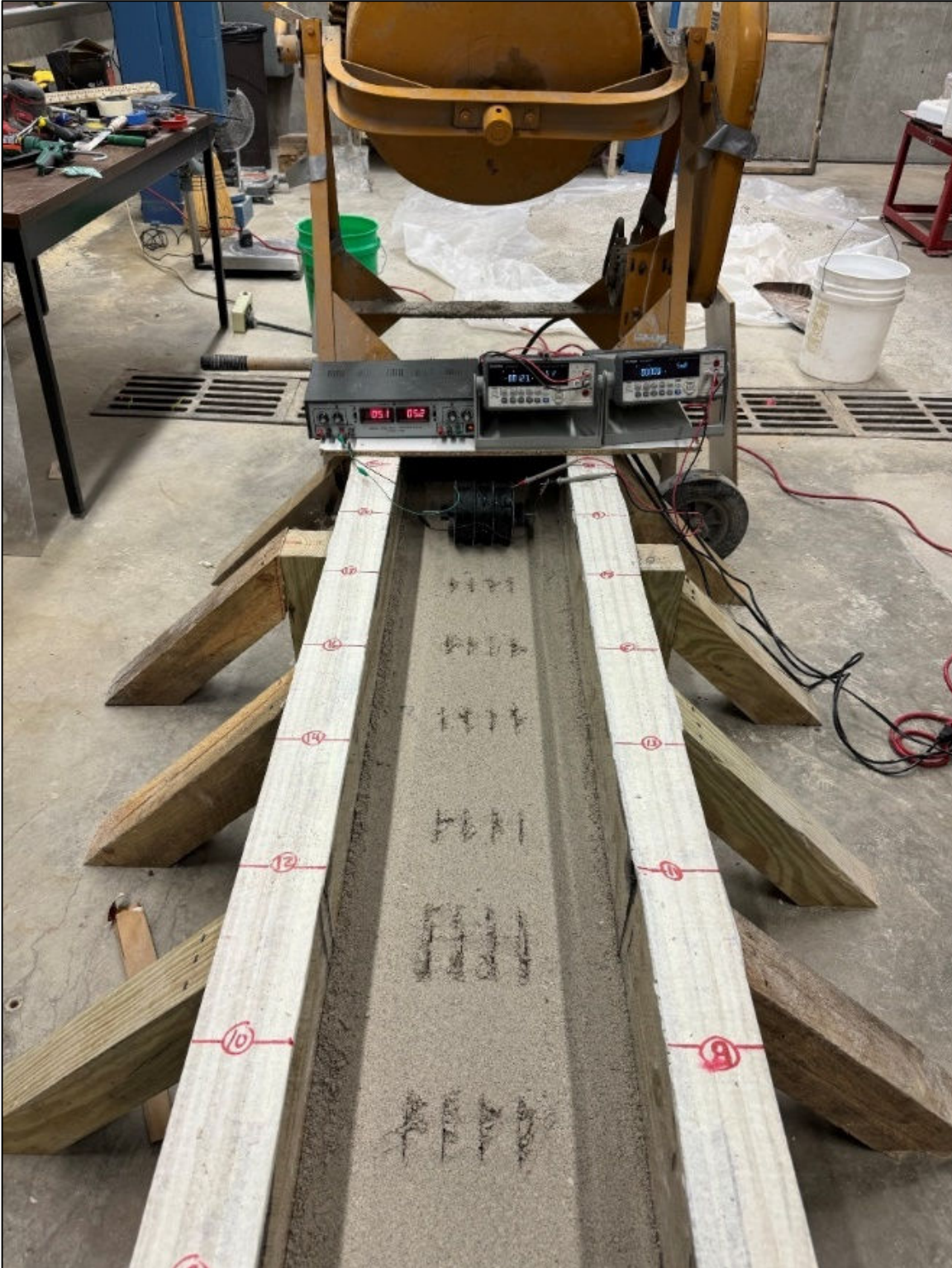
a) Single-Layer Sand Compaction System for ER Testing
