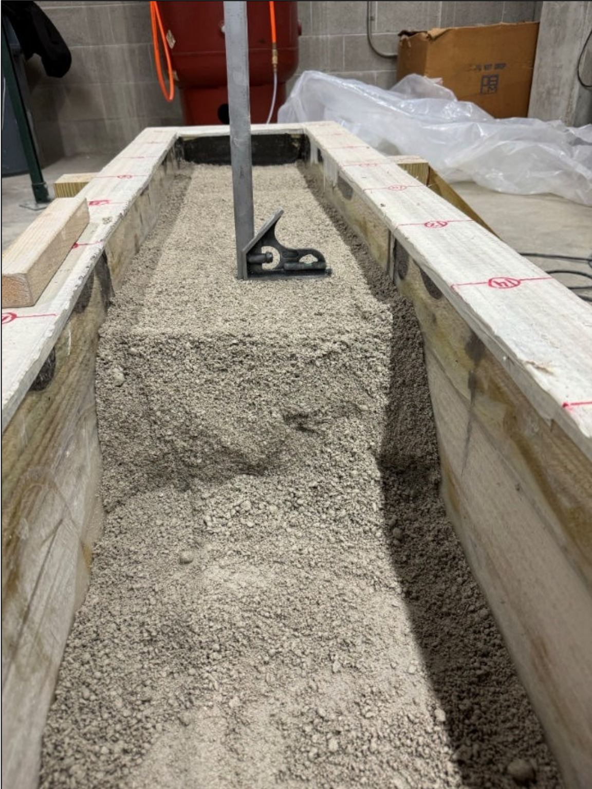
b) Two-Layer Sand Compaction System for ER Testing Figure 26: Comparison of Single- and Two-Layer Compaction Systems
