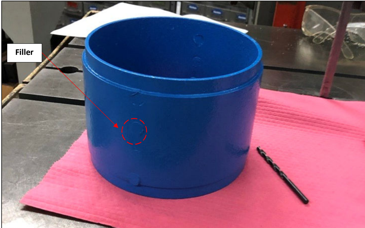
a) Epoxy-coated Proctor mold with four holes on each side with plastic filler
