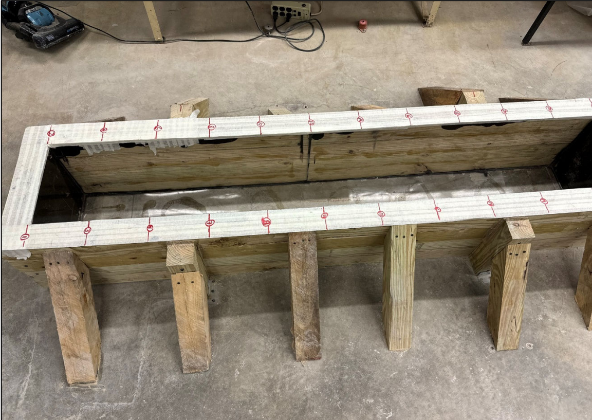
b) View of the Testing Container with Lateral Reinforcement
