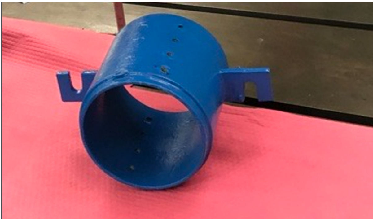
b) Four holes drilled through the plastic filler
